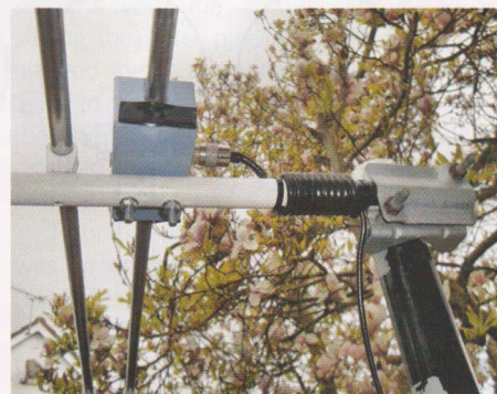
PHOTO 4: G3NKX antenna feed arrangement.
