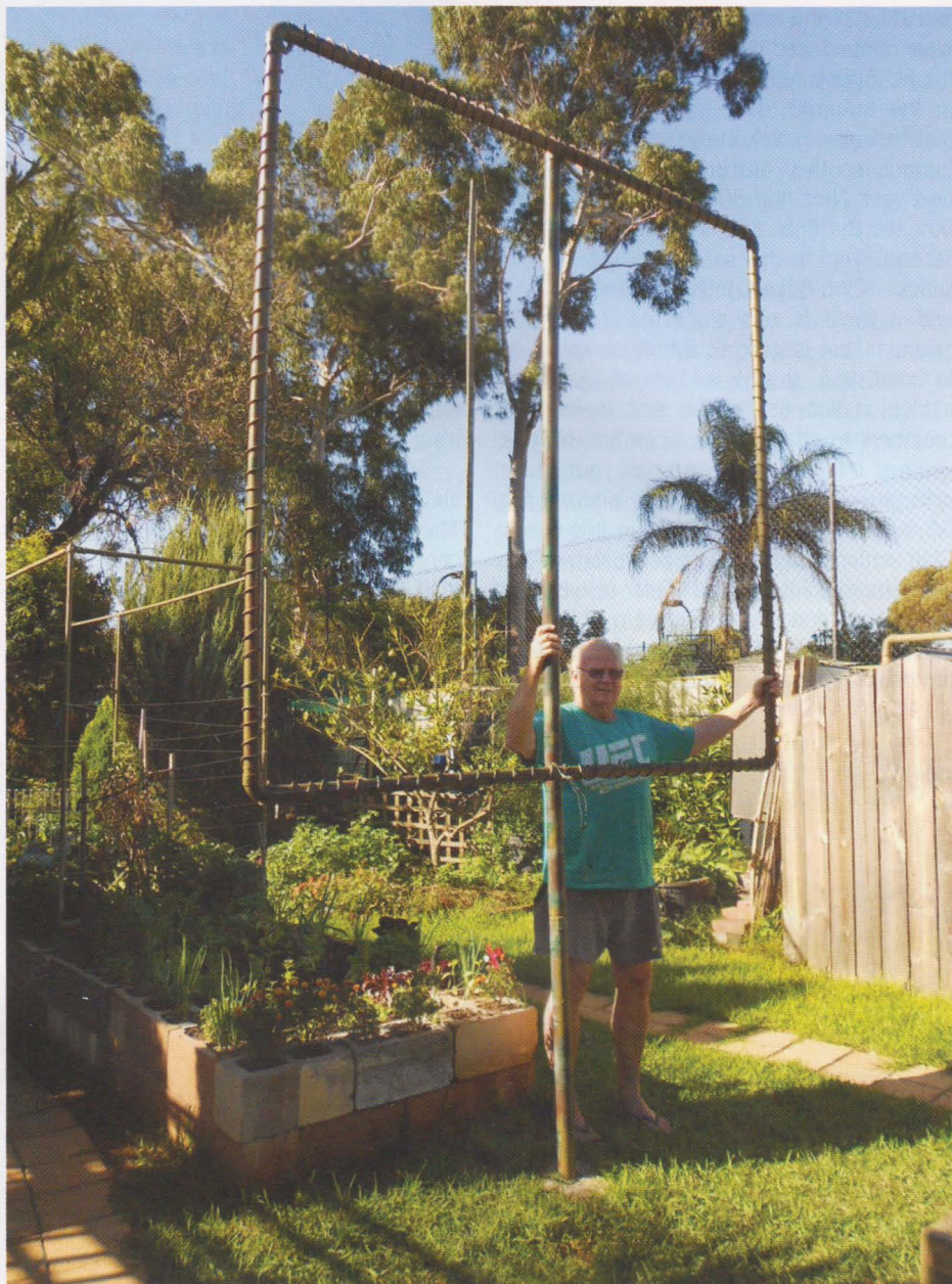
PHOTO 1: Finished antenna, with the author for scale.
