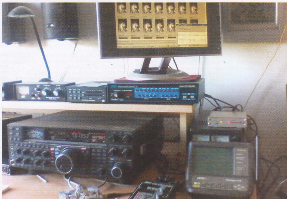
PHOTO 2: FT-2000, Pakratt PK-232 tnc, R2ZX receiver and Davis Vantage VUE weather console.
