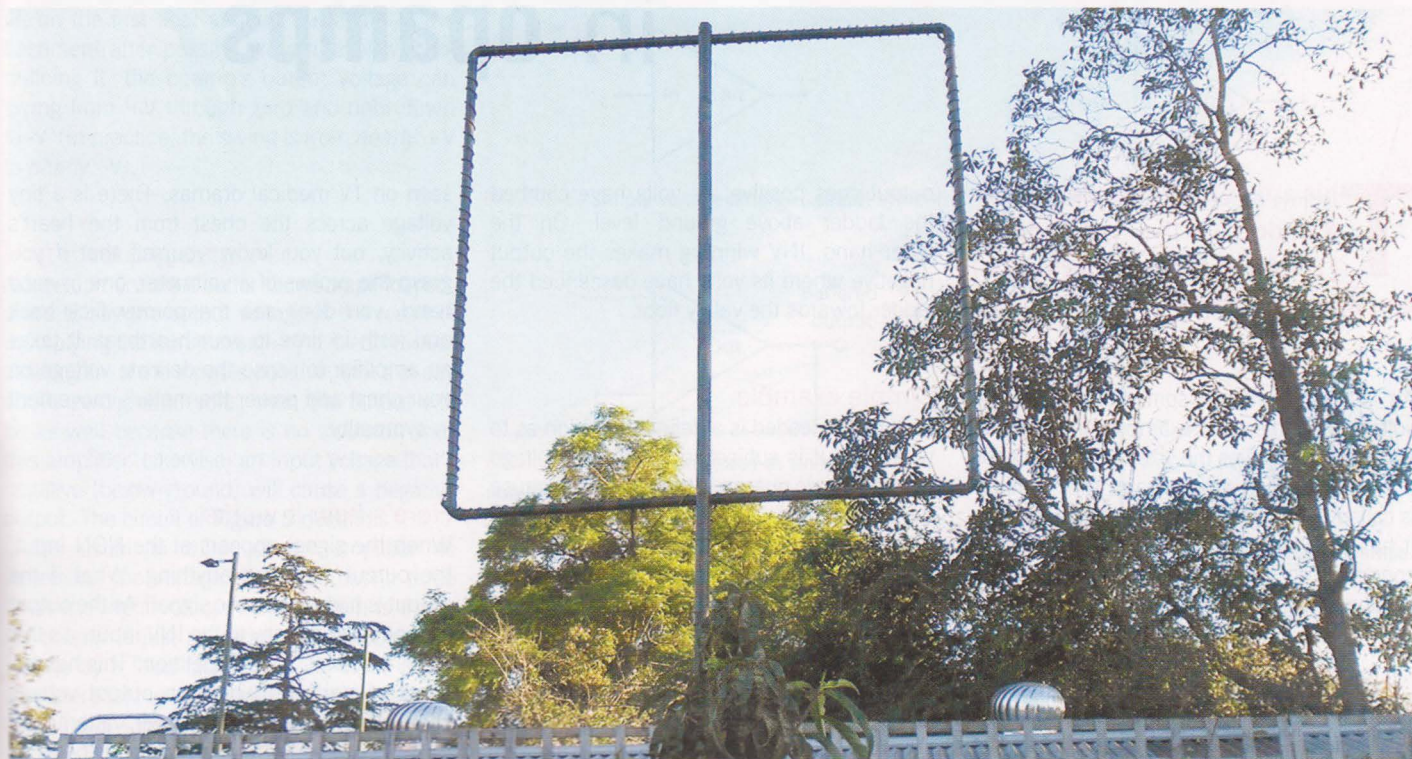
PHOTO 7: Completed loop on top of its timber mast.
