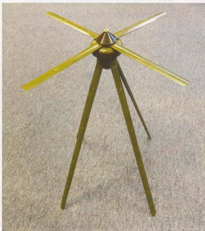
PHOTO 2: MORHE's novel discone antenna unfolded.
