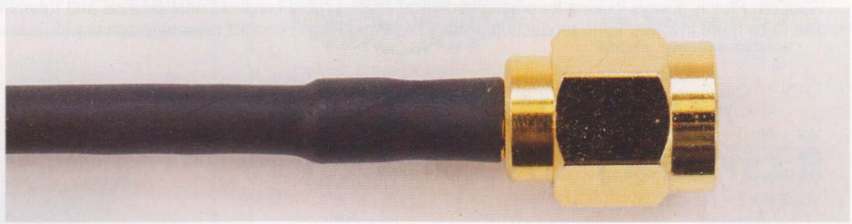
PHOTO 10: The completed termination.
