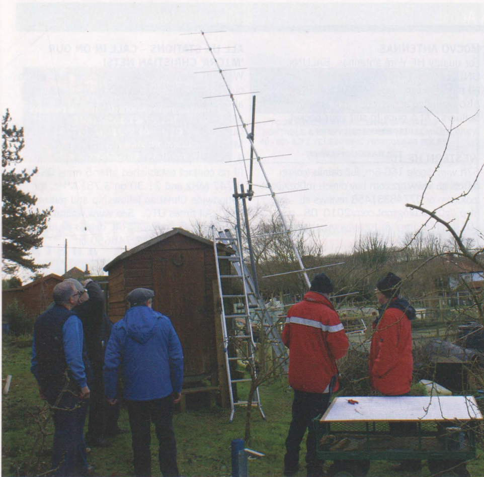
Norfolk Coast ARS has continued their experimentation with EME by constructing a 12-element 2m Yagi – on an 8m boom. Here it is shown on the simple manual pan/tilt arrangement that is located on a shed – on an allotment adjoining the club's facility. The location gives a clear view of the horizon from due south to west – and now it is just a case of waiting for a Thursday when the moon is in the right position during the club's meeting.
