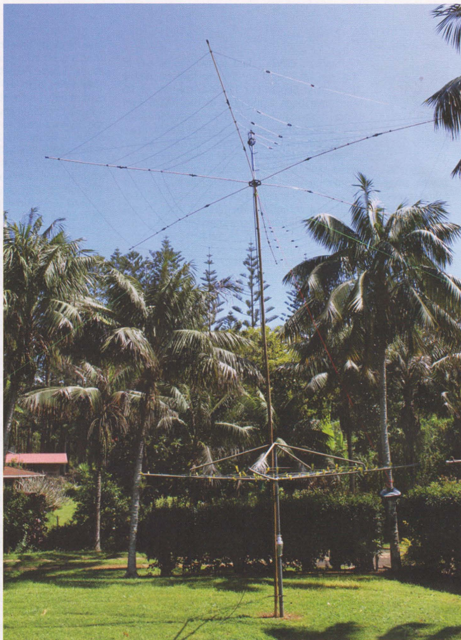
The team used a rotary clothes line and bamboo to support one of their hex beams.
