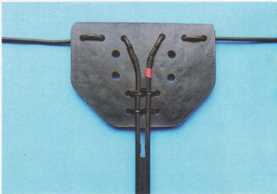
PHOTO 1: The dipole centre used for the doublet antenna, made from a small sheet of uPVC.
