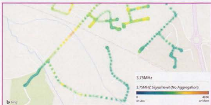
FIGURE 2: Heatmap for Guardband between D1 and U1 note blue levels as no VDSL at this frequency.
