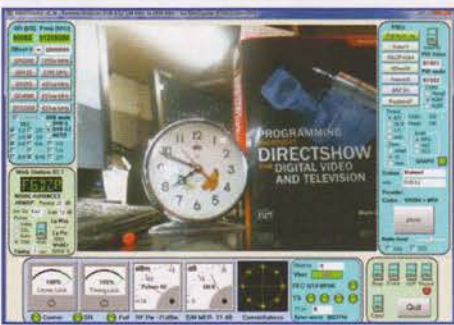
FIGURE 1: MiniTioune 0.7b demodulating DATV at 88kS/s. (Image: F6DZP).
