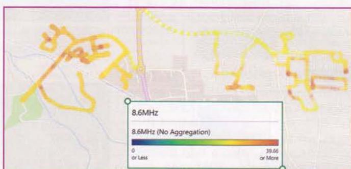
FIGURE 5: Heatmap bottom of Upstream 2 band usually most common source of RFI.
