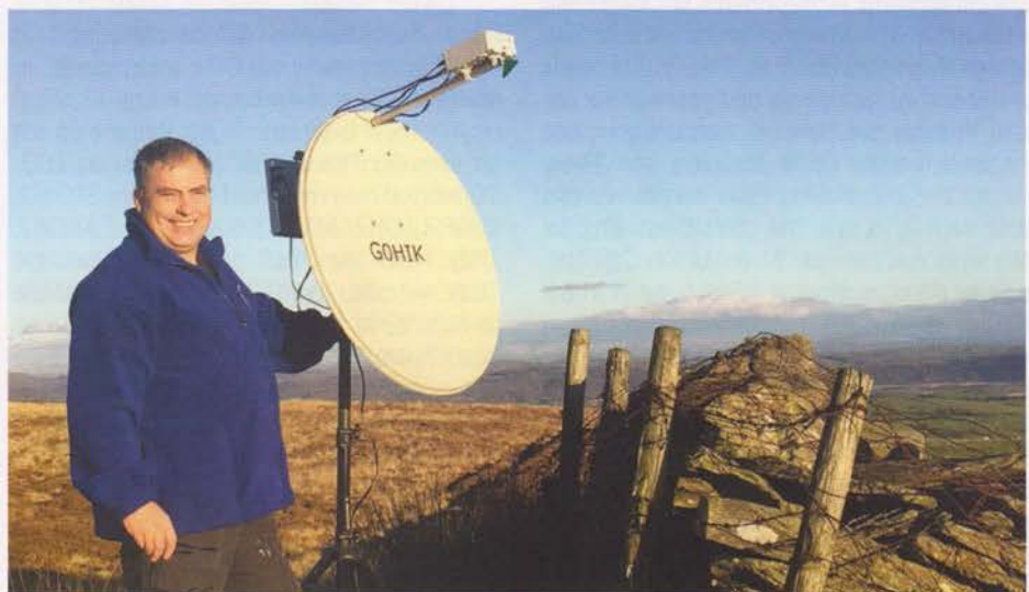
PHOTO 2: GOHIK with his 5.6GHz FM ATV receiver. Note the tiny PCB log periodic at the feedpoint.
