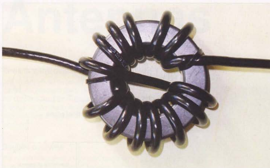
PHOTO 3: A 1:1 broadband balun based on the W1JR design using 12 turns of coaxial cable wound onto a FT240-31 core.
