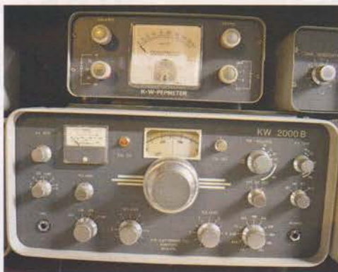
The most popular transceiver of all, the KW2000B, with the very rare 2 tone SSB PEP meter. Courtesy G3UGF.
