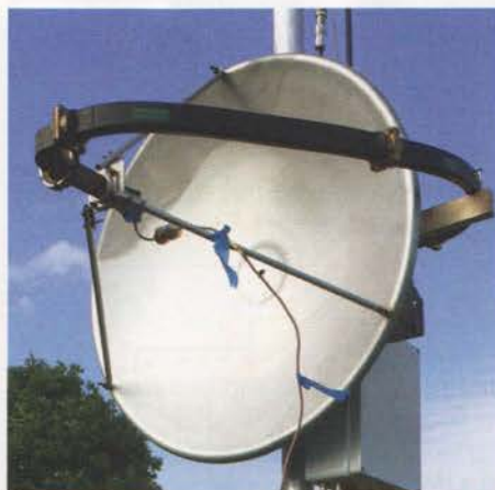
PHOTO 6: 10GHz dish with 5.6GHz dipole feed.
