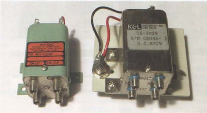
PHOTO 8: Typical suitable changeover relays. Those with four RF connectors are 'transfer' relays, which are also suitable for Tx/Rx changeover use.
