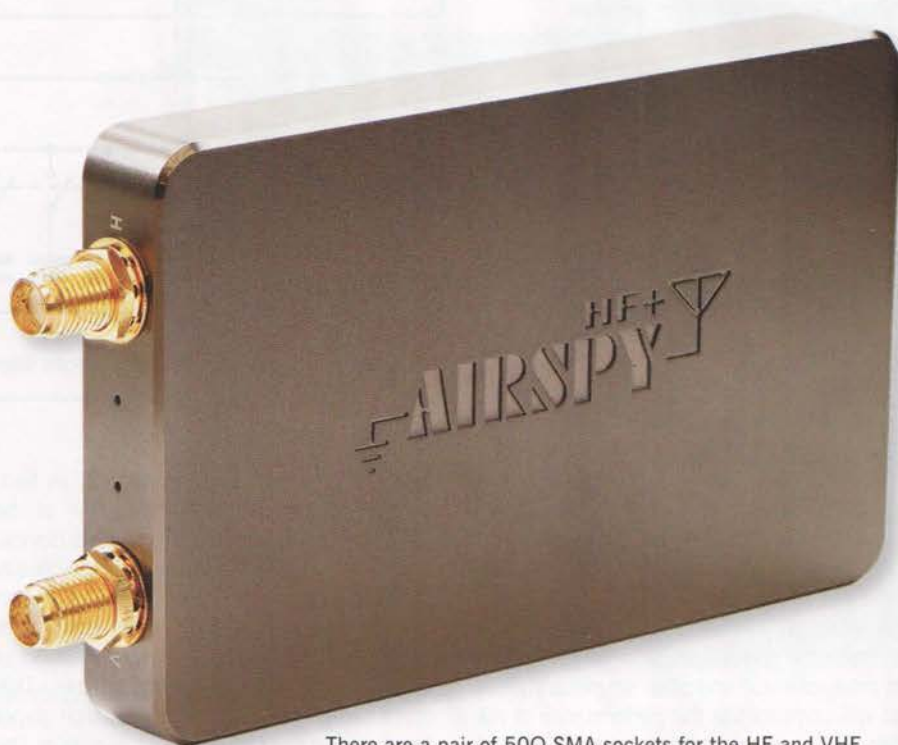
There are a pair of 50Ω SMA sockets for the HF and VHF antennas.
