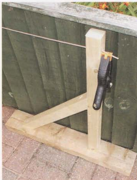
PHOTO 3: End of wire supported by a custom-made wooden support. The wire passes through a hole in the upright and is retained under tension using a spring clamp.
