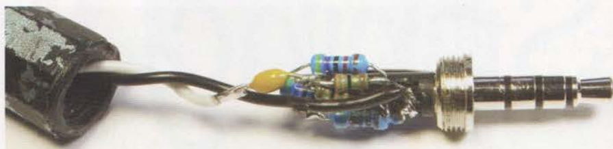
PHOTO 1: The components of Figure 1 fitted tightly into the barrel of the jack plug. A plastic barrel must be used as the outer shell of the jack is the microphone input, not ground.
