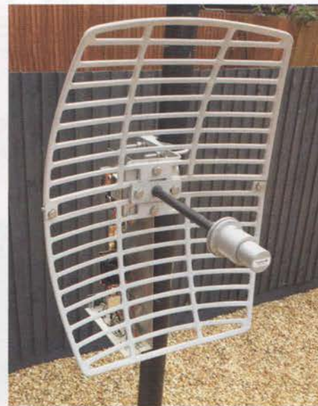
PHOTO 4: Hyperlink Technologies HG5 827G 27dBi 5.8GHz grid dish.
