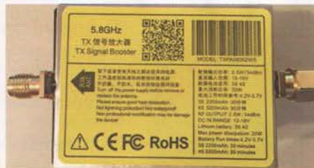
PHOTO 9: 2.5W 5.8GHz power amplifier.
