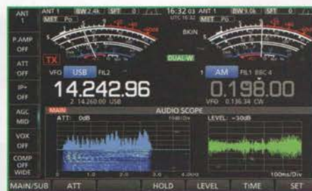
PHOTO 11: The audio scope display.
