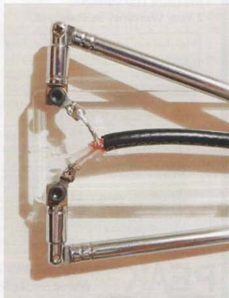
PHOTO 2: Mounting and connecting the elements.
