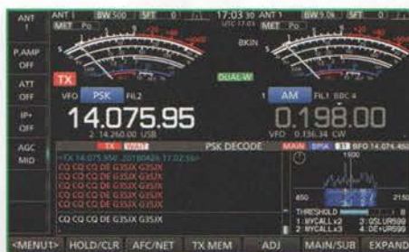
PHOTO 10: IC-7610 PSK decoder display.
