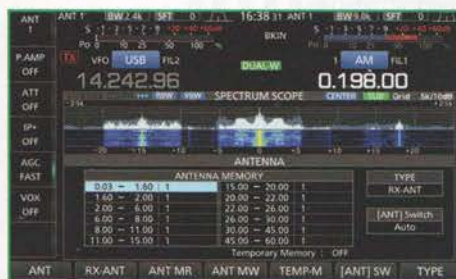
PHOTO 9: Antenna memory display and 'mini-scope' mode.
