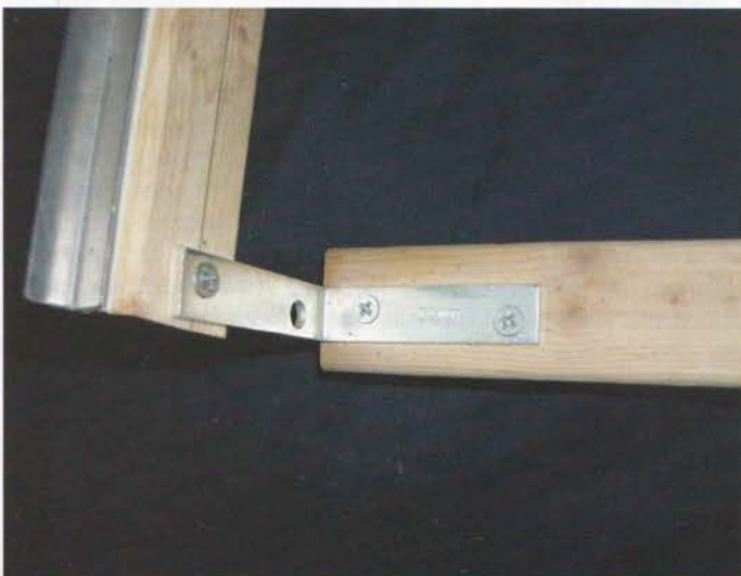
PHOTO 3: One of the brackets that elevates the front. The rear is similar, but lower. The L-shaped aluminium strip can be seen on the extreme left.
