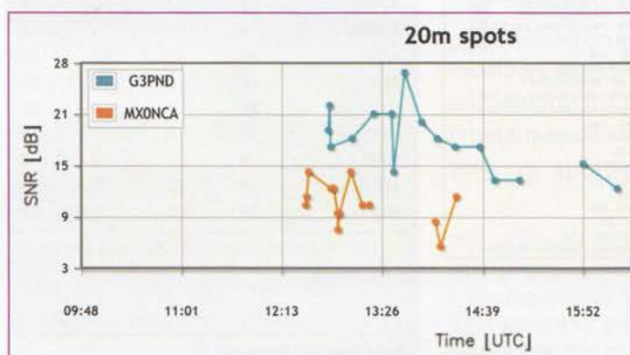
FIGURE 5: Results from the cubical quad test, W7ZI beacon.
