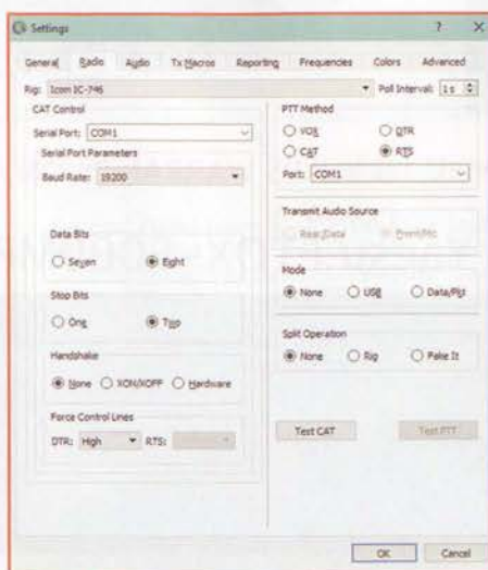
FIGURE 2: The WSJT software setup screen showing the settings needed to use the RS-232 to CI-V interface.
