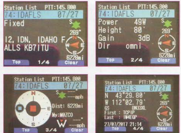
FIGURE 3: Screenshots from the Kenwood handheld of packet received from IDAFLS in Idaho, USA.
