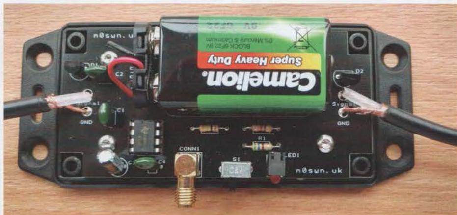
PHOTO 1: The fully developed PCB mounted on the lid of its box, showing the coax connections.
