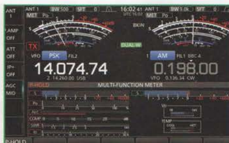
PHOTO 6: The multi-function meter displays the various transmit functions.
