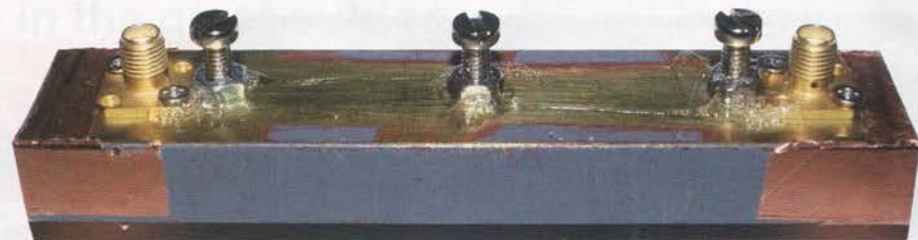
PHOTO 1: 3.4GHz evanescent mode bandpass filter.
