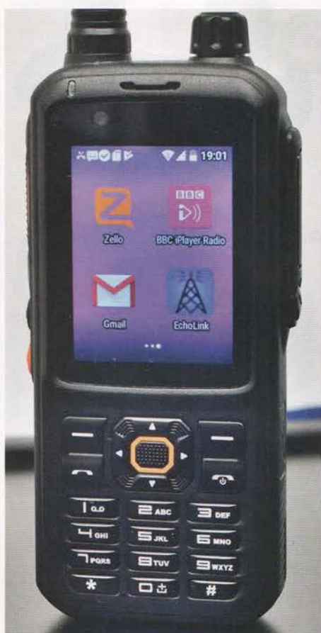
Underneath everything, the T320 is an Android device that runs standard apps.
