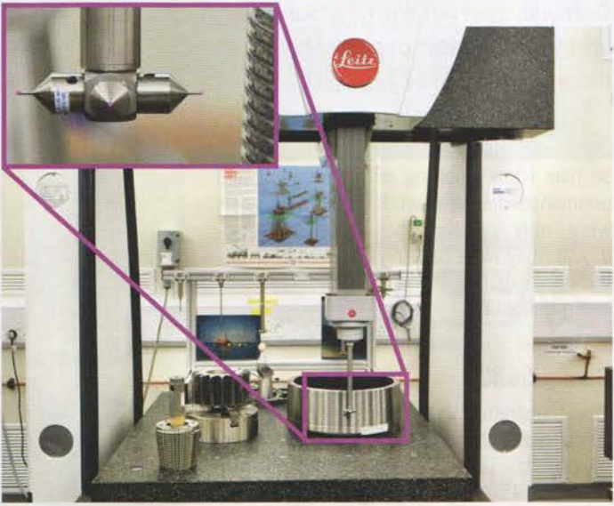
Ruby spheres of <1mm dia are the probes in this robotic precision measuring device, which manages wavelength-of-light-class accuracy in a volume of some 1.5m³. The machine is over 3m high and contains tonnes of granite.
