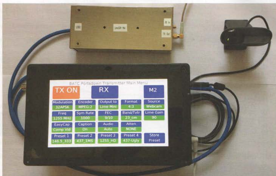
PHOTO 2: Portsdown transmitter with 7 inch touchscreen, webcam and Lime SDR Mini.
