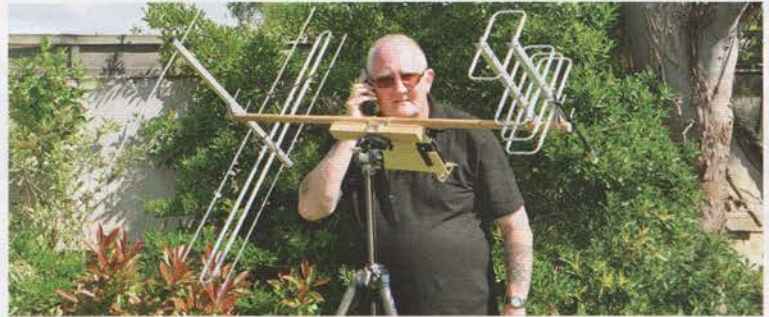
At the May meeting of Thames Amateur Radio Group, Mark MOIEO, gave a presentation on amateur satellites. He showed how mounting VHF and UHF antennas on a rod and tripod overcomes the limitation of only have two hands when needing to hold multiple bits of kit for the uplink and downlink. The wooden plinth in the middle is where the receiving radio is clipped. Mark's talk included a live demo on satellite tracking, accessing pass information from the AMSAT website, followed by a live demonstration of receiving a satellite communication from John, MOJRW in the car park. The next step is a Satellite field day at Hadleigh Country Park to attract club members and members of the public.
