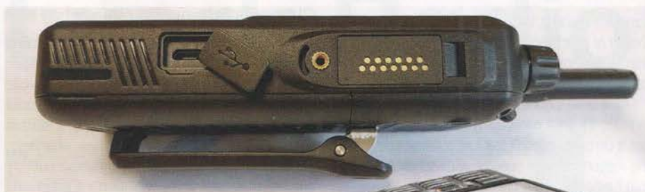
A captive cover conceals the micro USB charger socket, contributing to the T320's IP54 rating. A removable panel (retained by a screw) covers the accessory port's gold contacts.
