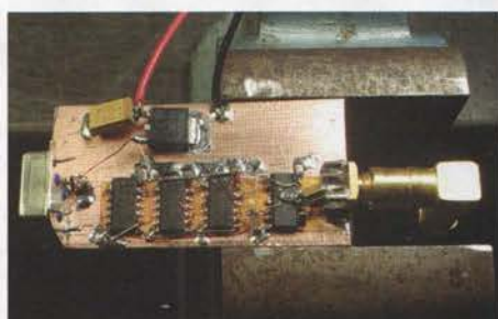
PHOTO 2: 23 BIT LFSR built using rats-nest construction.
