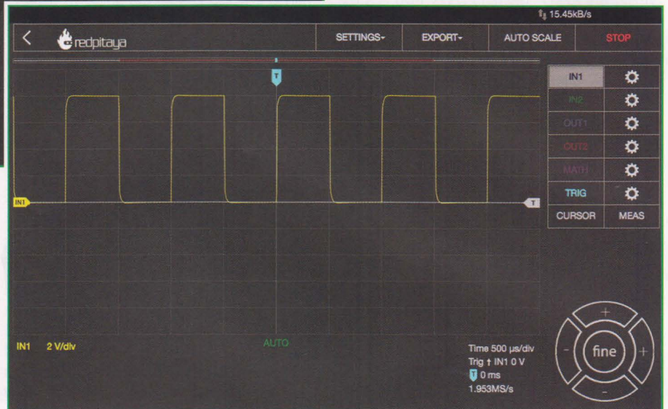
FIGURE 2: A waveform displayed on computer screen from the STEMLab oscilloscope. (NB some parts of this image have been enlarged so they appear more clearly here in print).
