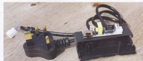
PHOTO 2: LED driver and mains plug for the LED sign.
