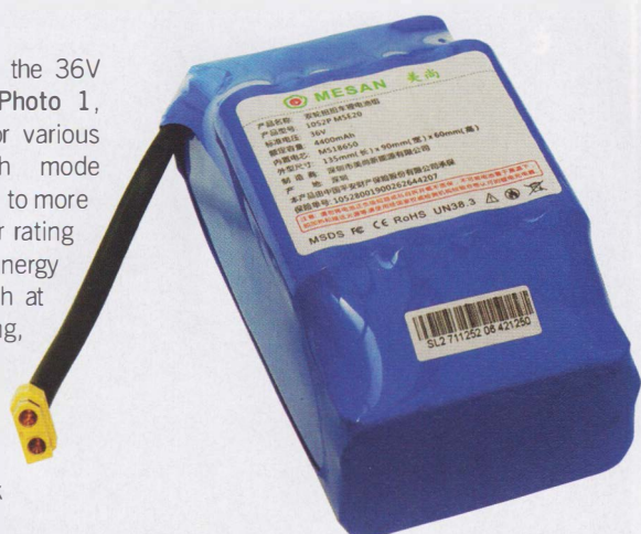
PHOTO 1: Ten-cell lithium battery pack purchased at a rally. At any reasonable state of charge its voltage would exceed the maximum input for most 'Simple Switcher' SMPSU devices.
