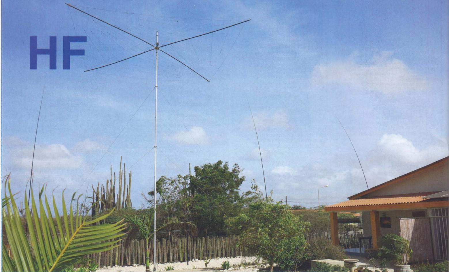
The PJ4DX QTH in Bonaire with 80m vertical, Spiderbeam, and two element phased array on 40m.
