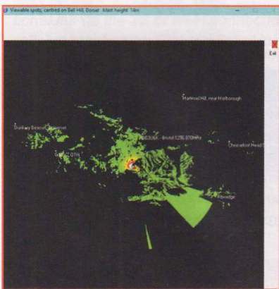
FIGURE 4: Plot of visible terrain from the same site. The colour corresponds to horizon angle, with black sections not visible. The cursor position reads out NGR, Locator, and the nearest site, allowing various high spots and line of sight paths to be discovered.
