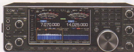
Rather than using any analogue mixers, the Icom IC-7610's leading-edge receivers directly sample the incoming RF at very high speed, downconverting digitally in an FPGA.
