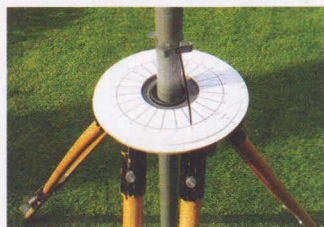
PHOTO 2: The protractor and pointer arrangement used during the measurements.
