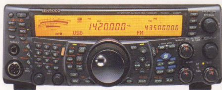
The DSP in Kenwood's TS-2000 operates on a 12kHz IF at the end of an otherwise traditional analogue superhet architecture.
