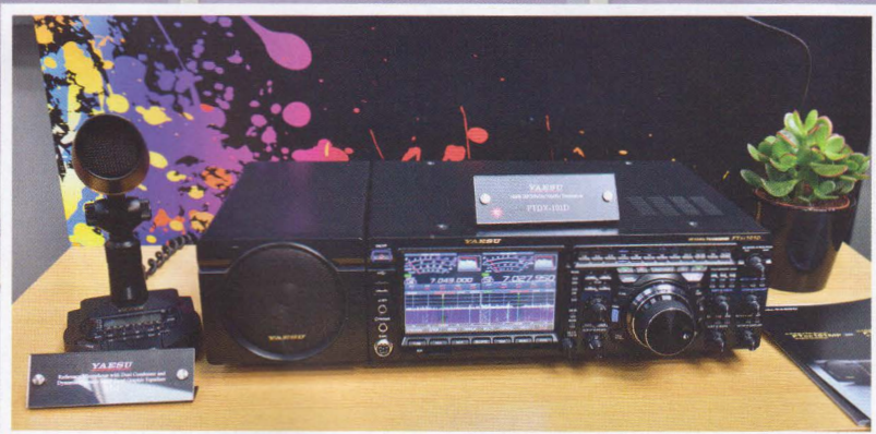
Yaesu showed their brand new 100W FTx101D all mode HF, 6m and 4m transceiver. Demonstrating their long commitment to amateur radio, they also showed a 1970s FT-101B and an FT-101ZD. Separately, on the RSGB QSL Bureau stand, was the historic, fabled and ultra-rare KW 2000D, courtesy of the National Radio Centre.
