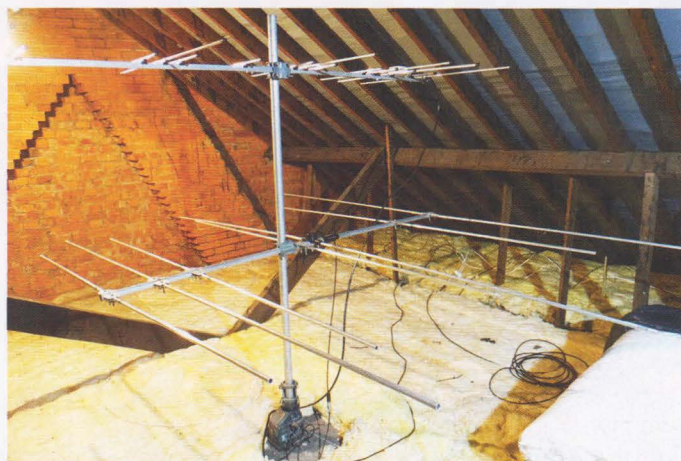
PHOTO 3: The 6m/4m dual-band Yagi beam featured in the September Antennas column in use in the loft at G4FOY's QTH.
