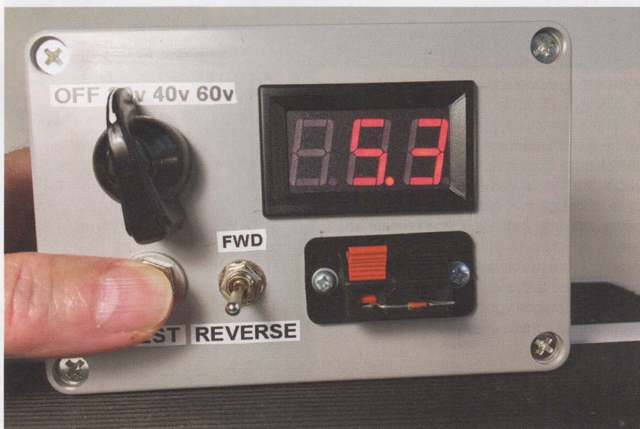
PHOTO 4: Testing a 5.3V Zener diode.
