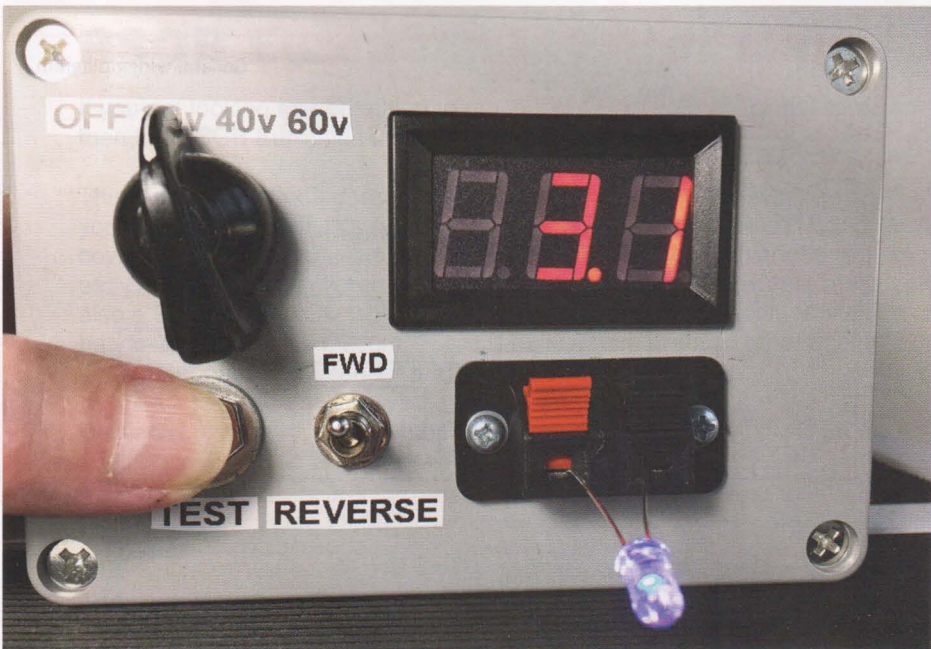
PHOTO 3: Typical test showing the 3.1V forward voltage of a blue LED.
