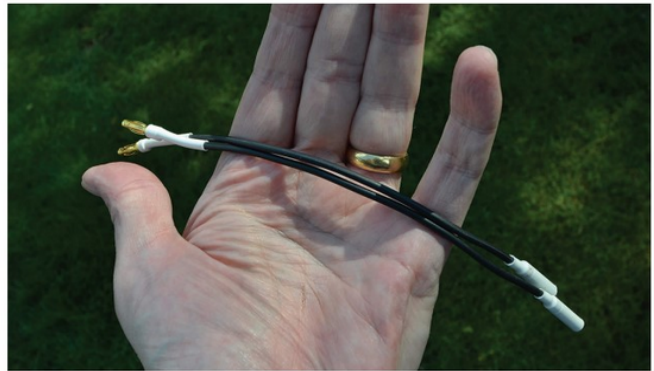
The antenna comes with an assorted of 'extenders' to move the resonant frequency down.
