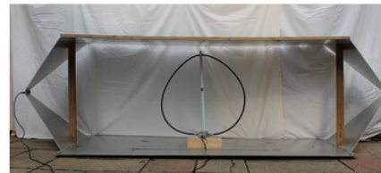
PHOTO 7: Calibrating a shielded loop antenna using a TEM Cell.
