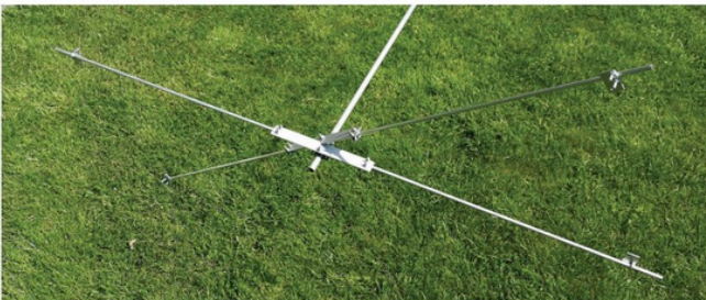
PHOTO 3: Two crossing tubes are attached to the end of every leg. They will support a copper wire frame 0.6m high and 1.2m wide.
