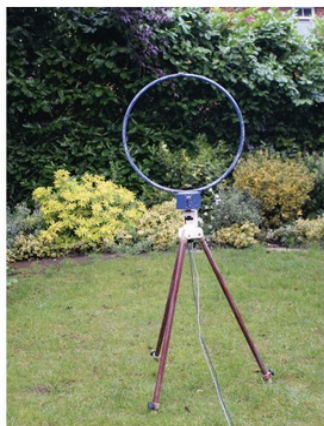
PHOTO 1: Schaffner-Chase HLA6120 active EMC measuring loop antenna, 9kHz–30MHz.
