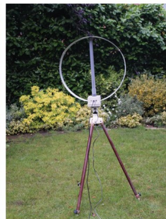
PHOTO 4: Active broadband or tuned loop antenna. Photos 1-4 are at approximately the same scale.
