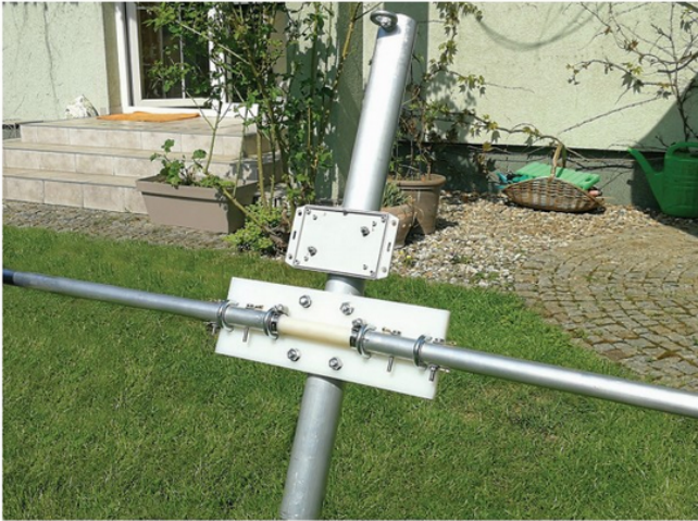
PHOTO 2: Central part of the antenna structure. A polyamide plate and rod as well as U-clamps were used to join the two legs of the doublet.
