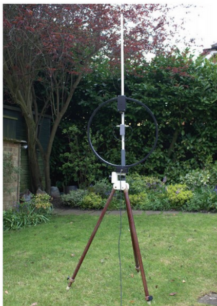
PHOTO 6: Calibrating a 'bicycle wheel loop' antenna using a crystal calibrator.
