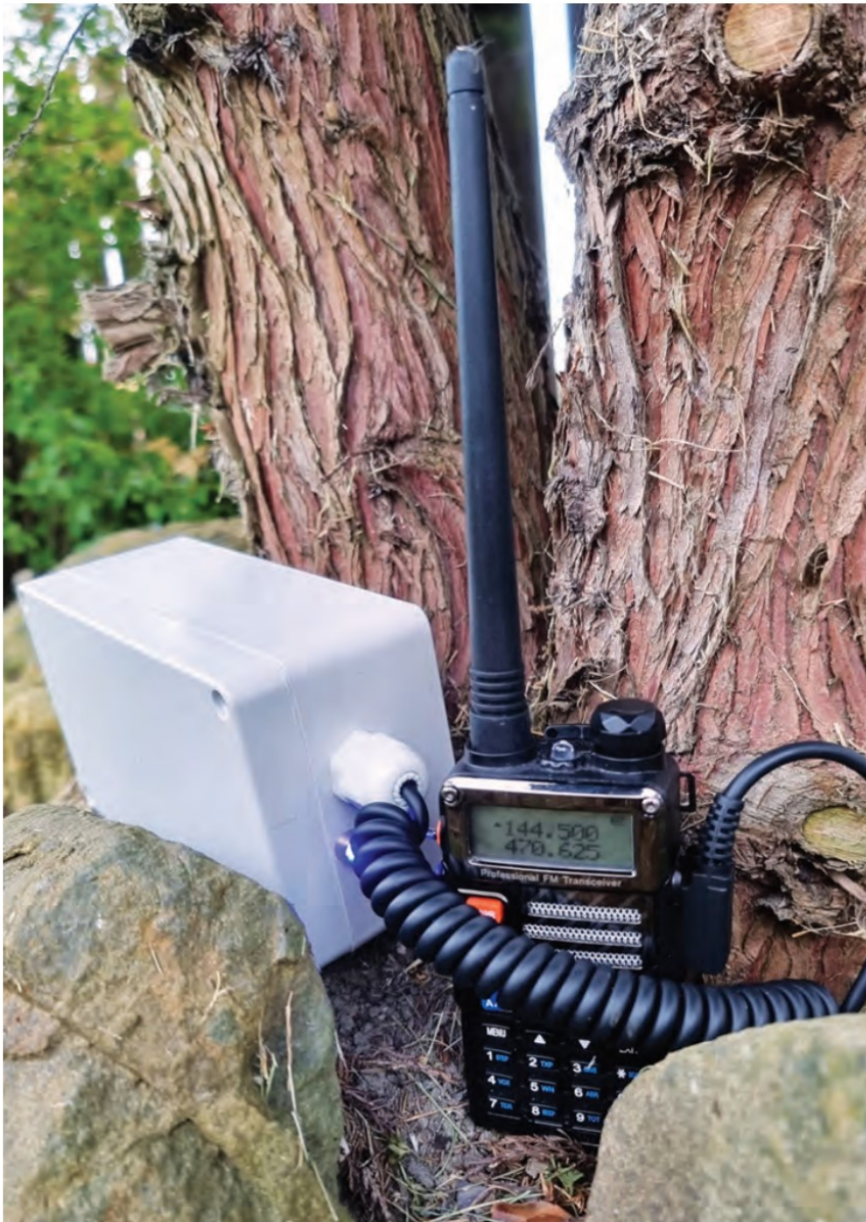
PHOTO 8: IP65 enclosure and UV5R hiding
