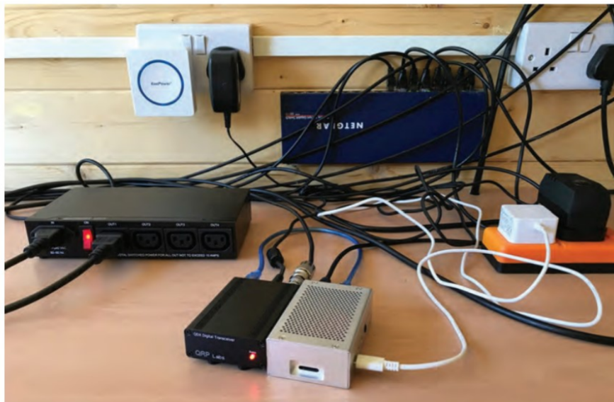
Photo 4. QRP Labs QDX inside its case, Raspberry Pi 4 powered from PoIP Switch.
