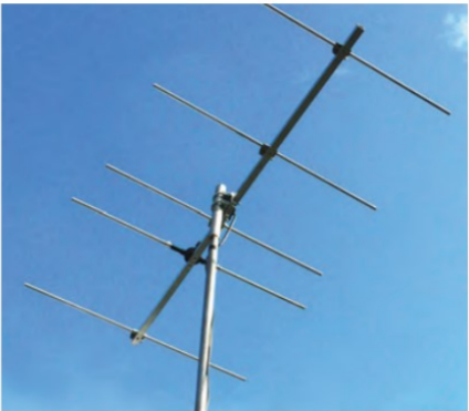
PHOTO 3: 5-element 2m Yagi beam using elements made from individual 12mm diameter aluminium tubes.
