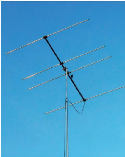
PHOTO 3: The 4-element Yagi beam array for the 4m band in use.
