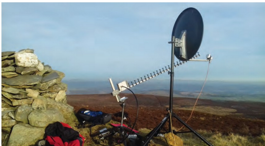
My first SOTA QO-100 experiments used a 25-ele Tonna Yagi and a Sky-type dish.
