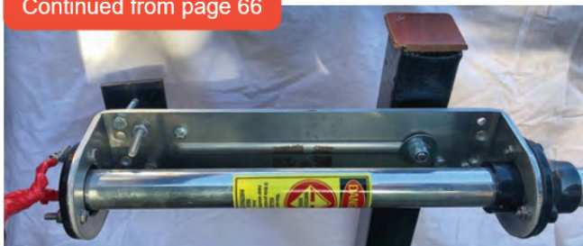
PHOTO 2: Antenna mount in luffed (down) position.
