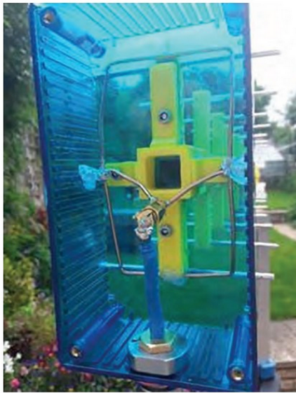
PHOTO 4: Feed mounted inside protective box.
