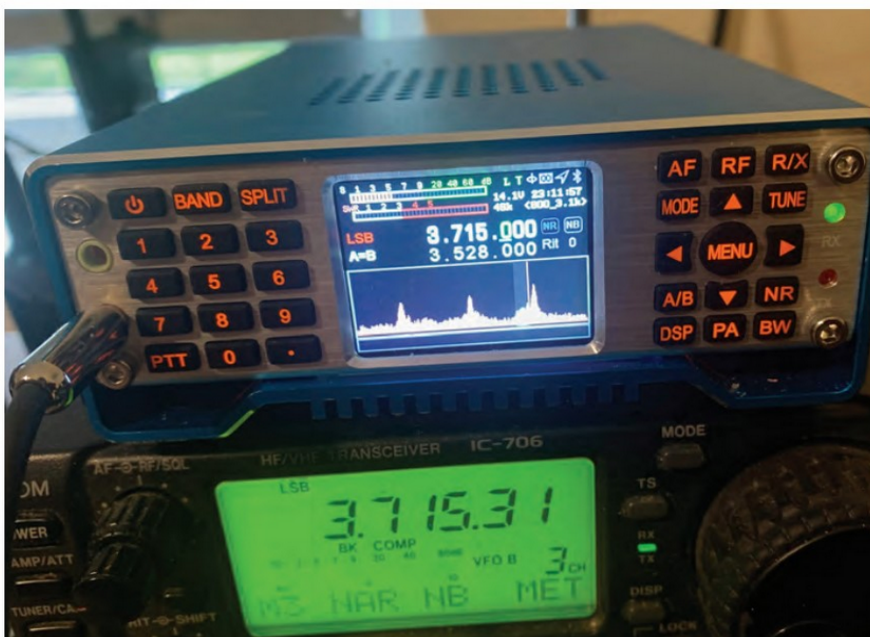
Ailunce is a relatively new name in the amateur market. The HS-2 is an SDR transceiver.
