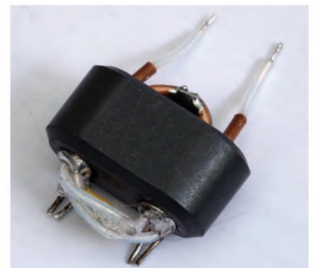
PHOTO 2: 1:3 turns ratio transformer using lengths of semi rigid coax.
