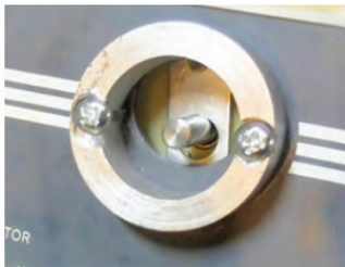
PHOTO 7: Recessed screws in the spacer showing the clamp behind the panel and the off-centre hole.
