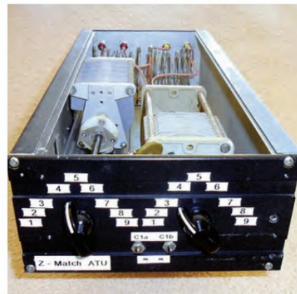
PHOTO 4: Front panel of G40JMI's Z-match ATU. Note the use of the numbered scales to record the setting for each band.
