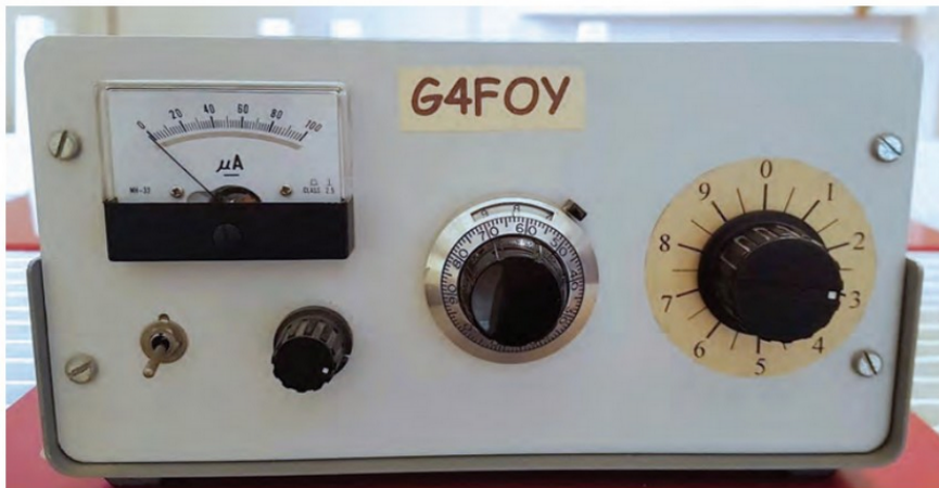
PHOTO 2: Front panel of G4FOY's T-network ATU. Note the use of the calibrated control for adjusting the roller-coaster inductor to indicate the setting for each band.
