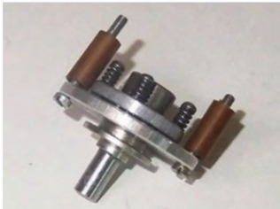
PHOTO 10: The clutch showing the grub screws and the 14mm spacers.
