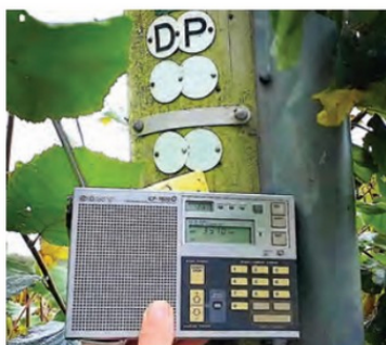
PHOTO 2: A telephone pole found to be radiating QRM on 3571kHz.
