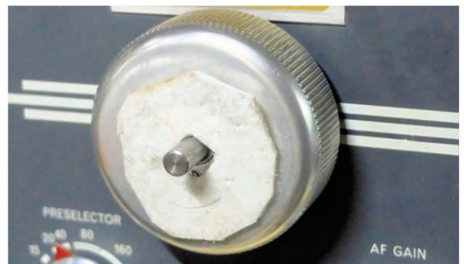
PHOTO 14: The felt disc between inner and outer controls.
