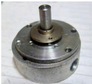
PHOTO 4: Reduction drive as removed.
