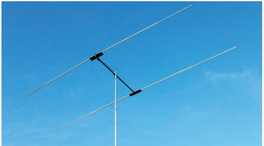
PHOTO 1: The 10m band 2-ele beam array in use.
