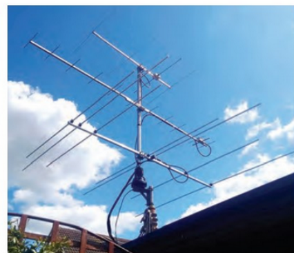
PHOTO 4: G8XIR's 6m/4m Yagi beam antenna mounted below his 70m and 2m Yagi beams on his pump up mast.
