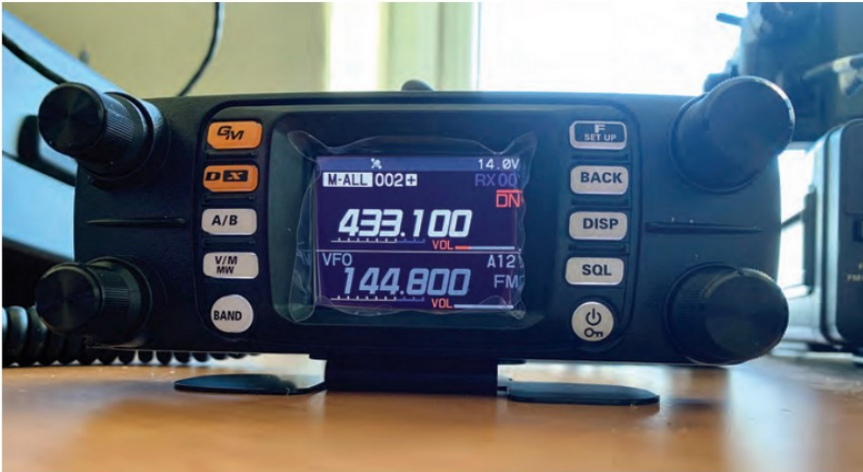
The Yaesu FT-M300 is a dual band transceiver, 144 and 430MHz bands.
