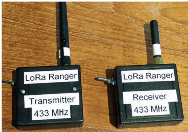
PHOTO 2: My prototype 433MHz range testers.
