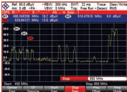
FIGURE 1: Spectrum plot of UHF TV band near a 4G base station.
