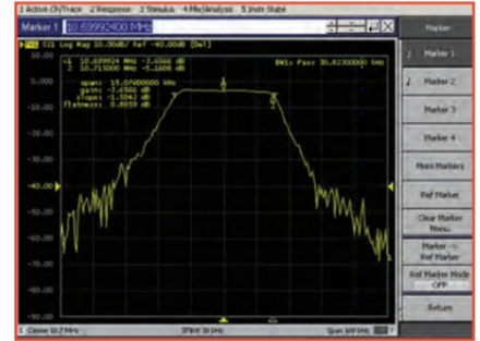
FIGURE 2: 10.7MHz IF filter response.
