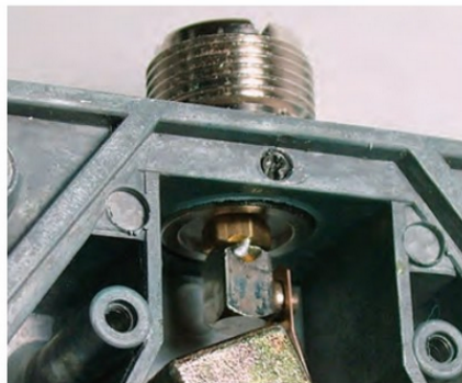
PHOTO 2: Coax switch with rotated contact.
