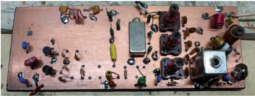
PHOTO 3: Front end, RF filter (with the RF cans removed), mixer and buffer amplifier.
