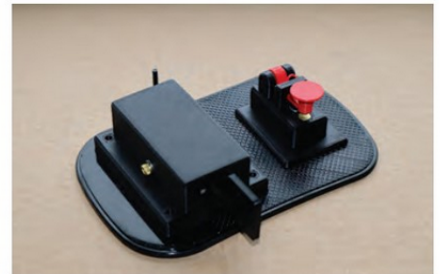
PHOTO 5: Using a gel pad to secure keys and paddles.
