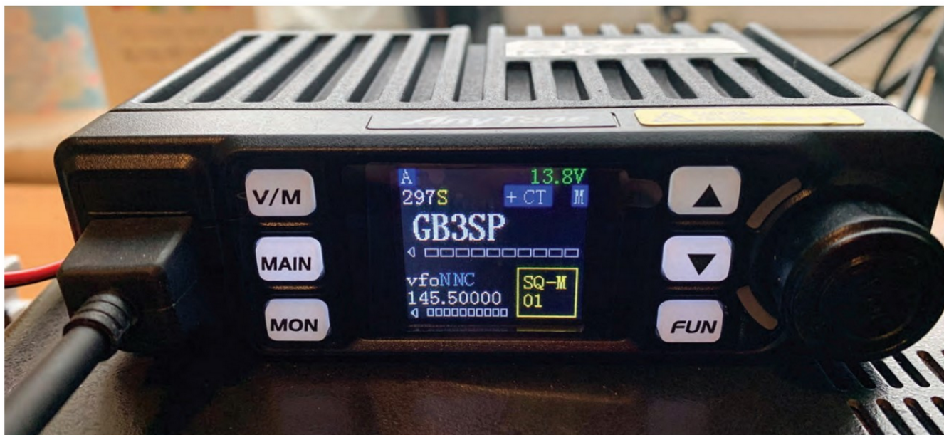
Measuring just 124mm (W) x 101mm (D) x 36mm (H) the Anytone AT-779UV is still a dual band VHF/UHF 25/10/5W transceiver.
