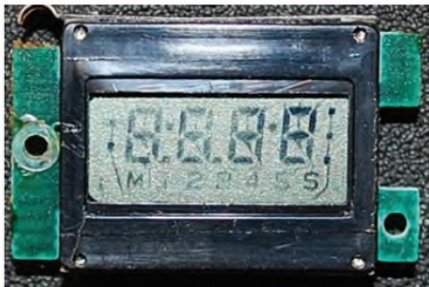
PHOTO 2: The original Standard C-58 display had deteriorated badly.
