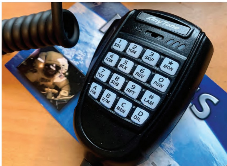
You can change the power level to high from the microphone control at the touch of the button.
