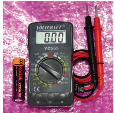
PHOTO 2: An inexpensive, pocket-size, 3\frac{1}{2} digit DMM with captive leads – ideal for many quick checks.
