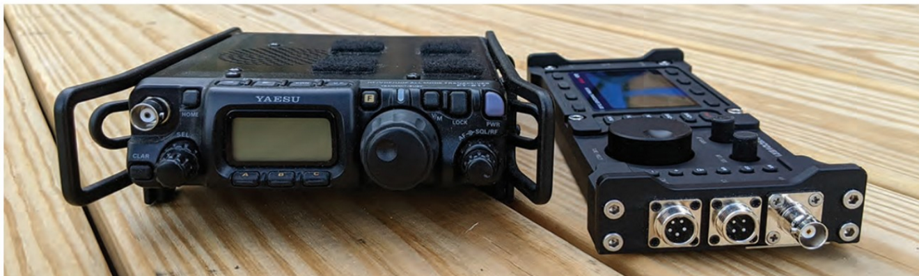
My Yaesu FT-817 next to the Discovery TX-500 showing the unusually small profile of the QRP transceiver.
