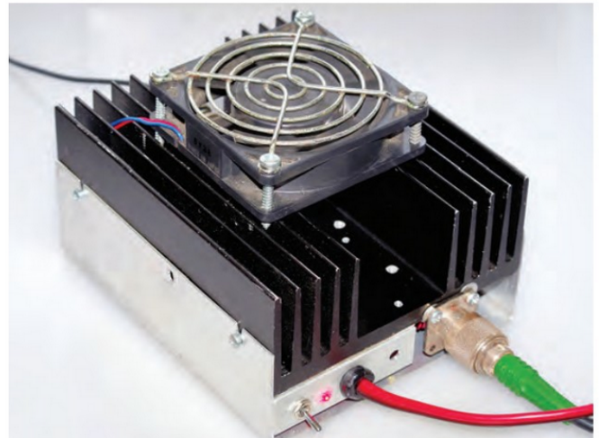
PHOTO 3: Finished amplifier showing heatsink and fan.
