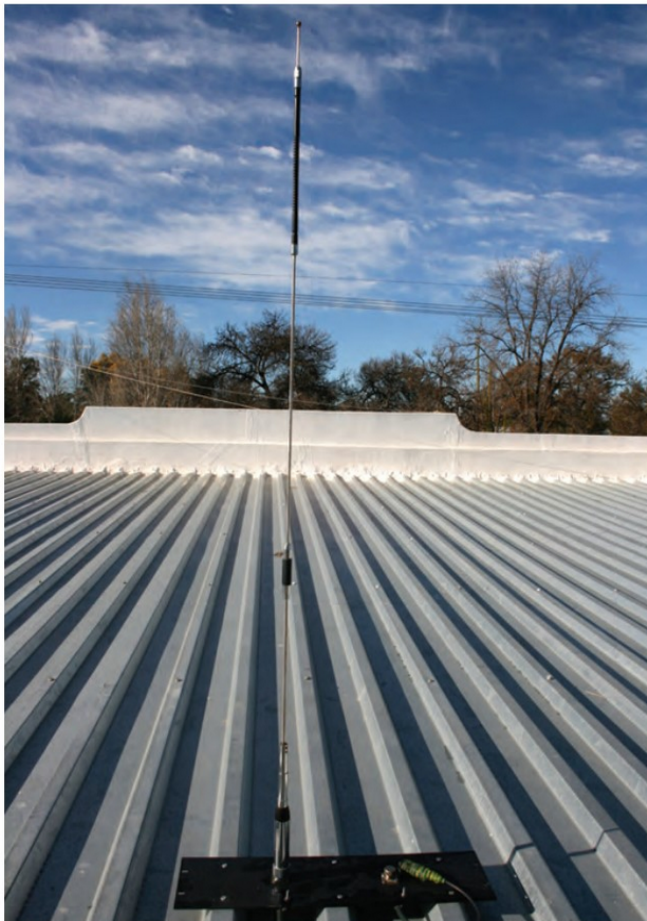
PHOTO 2: A simple mobile antenna is all I needed to listen to the ISS using my FT-8900.
