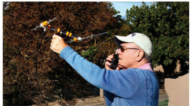
PHOTO 4: A compact HB9CV antenna significantly improved my signal into the ISS, but still only needing 5W from the handie.
