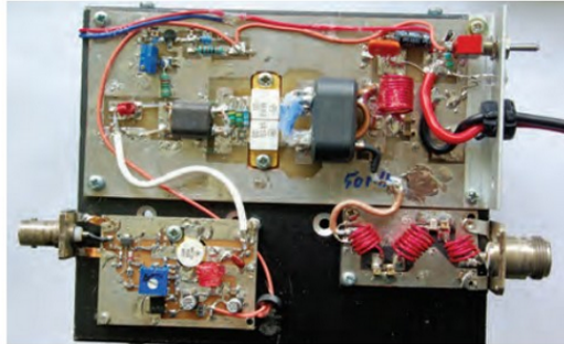
PHOTO 2: The 50MHz power amp's three units: the 5W driver, main power amplifier and output filter with L/C matching.
