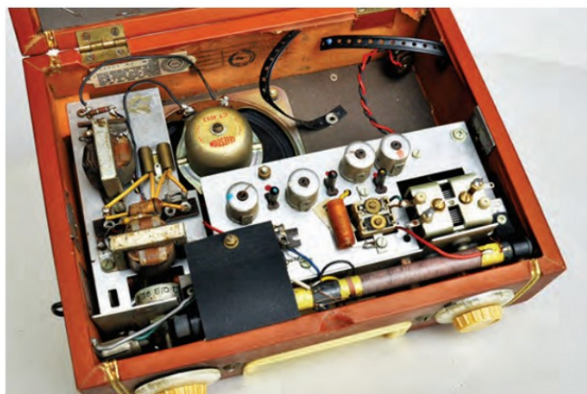
PHOTO 4: The double aluminium chassis of the Ever Ready 'Sky Leader'. Later models made use of printed circuit boards.
