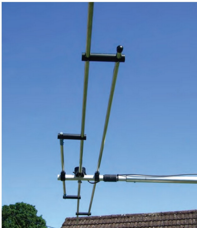
PHOTO 3: G4JBE's 6m/4m/2m tri-band antenna under test.
