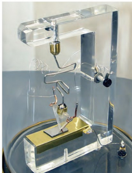
PHOTO 1: Replica model of the first transistor. Image: 'Mister rf' via Wikimedia Commons, CC BY-SA 4.0.
