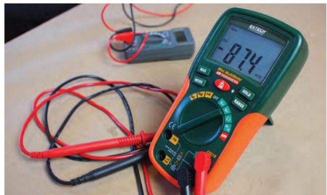
PHOTO 3: This auto-ranging 3½ digit DMM also includes a non-contact infrared thermometer. (Photo courtesy Becky Stern via Wikimedia Commons, CC BY-SA 2.0).
