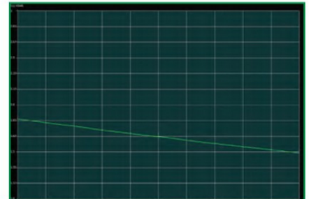
On 17m the SWR good have been improved by making the element a little longer.
