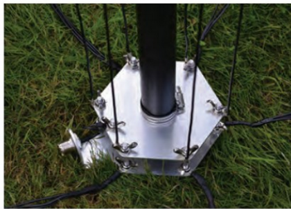
The driven and ground plates with wingnuts and driven elements attached.
