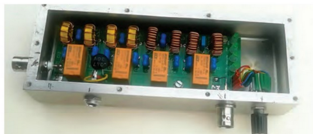
PHOTO 6: eBay-sourced 5-pole switchable filter bank.
