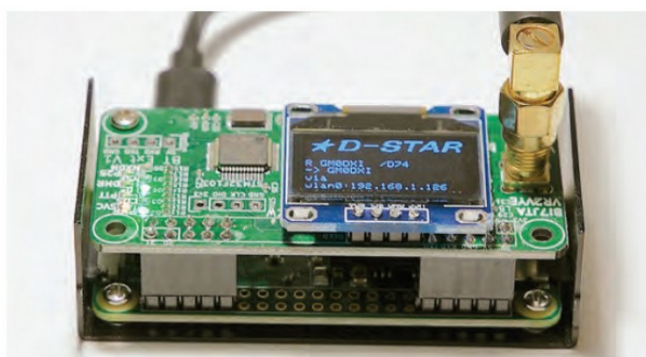
PHOTO 2: The Retevis MMDVM hotspot is a 'HAT' on a Raspberry Pi Zero W.
