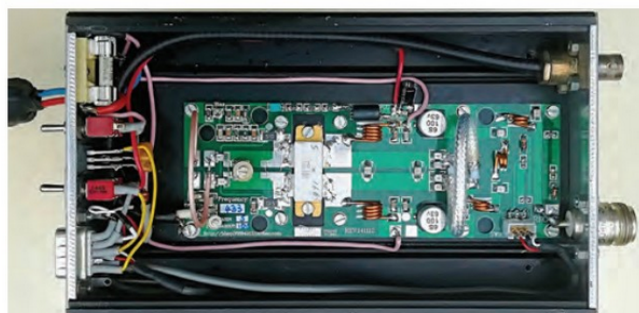
PHOTO 8: eBay-sourced '100W' 70cm amplifier housed in a recycled case.
