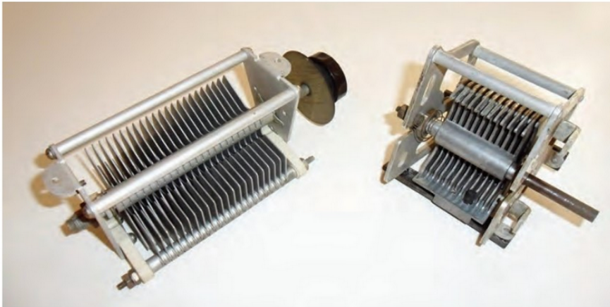
PHOTO 2: Two examples of variable capacitors able to withstand higher RF voltages.
