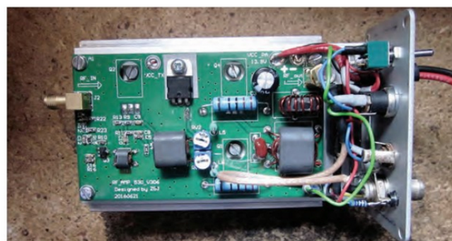
PHOTO 5: eBay-sourced '45W' HF amplifier that required filtering.
