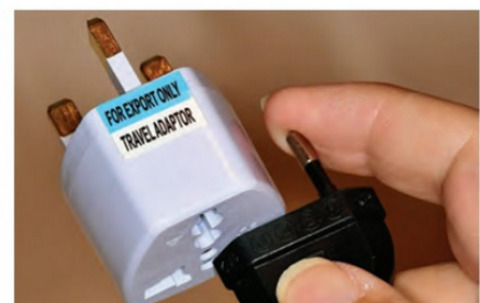
PHOTO 6: An unsafe 2-pin adaptor with partially sleeved earth pin, no fuse and unshuttered contacts that poses a shock risk.
