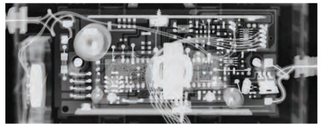
PHOTO 3: X-ray view of a very similar battery charger (courtesy G1MFG).
