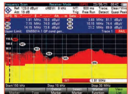
FIGURE 2: Conducted emissions from a battery charger up to 30MHz.
