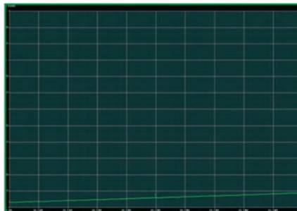
A scan using my nanoVNA shows a low SWR across 30 metres.
