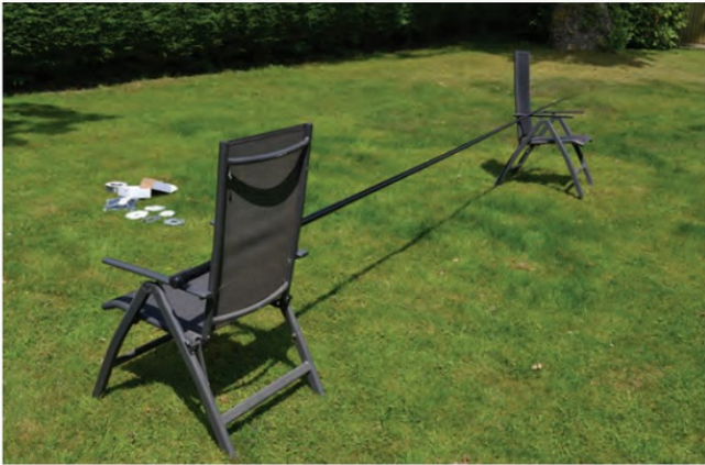
Callum recommends supporting the antenna on two chairs while you build it.
