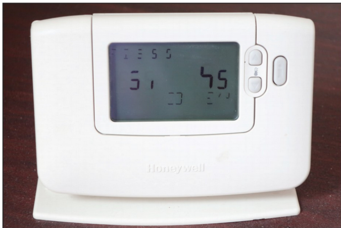
PHOTO 1: Honeywell Thermostat with faded display.
