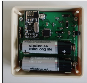
PHOTO 4: Internal view of finished sensor boxed in a commercial enclosure.
