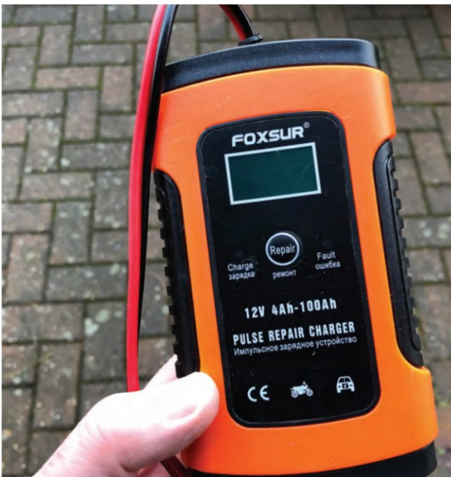
PHOTO 6: This battery charger turned out to be the source of the QRM.
