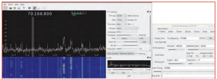
FIGURE 1: Screenshot of GQRx receiving 70MHz during a UKAC contest (left) plus my GNUradio transmit software (right).
