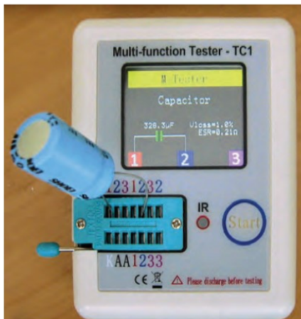
PHOTO 4: How an electrolytic capacitor shapes up, including measuring its ESR.
