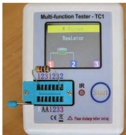
PHOTO 3: A 1kΩ resistor may not be a challenge but confirms you've read the colour code correctly.
