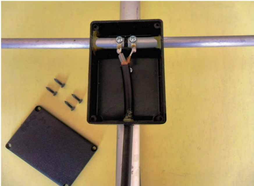
PHOTO 2: Homemade dipole centre used for the 70cm band Yagi beam array made using an ABS box, aluminium tubes and a plastic rod.
