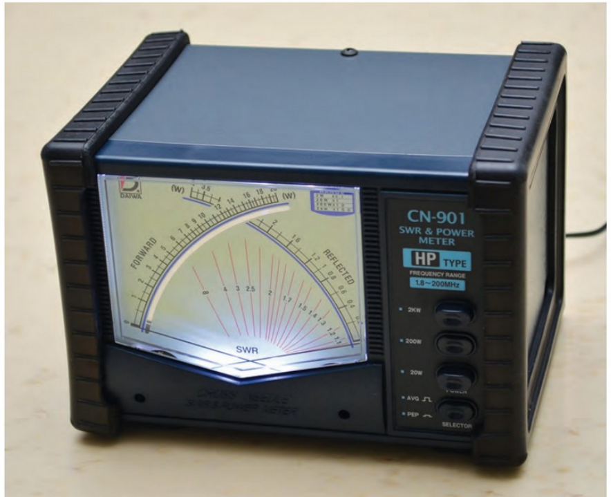
The meter reads the SWR at the point the meter needles cross.
