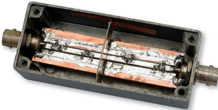
PHOTO 2: Practical implementation of Figure 1. Constructed using 0805 SMT resistors on microstrip. There is a continuous ground plane on the rear with copper foil wrapped round the long edges connecting the top grounding area to this.
