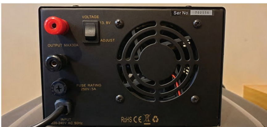
The back of the Sharman multiCOM SM-30II switch-mode power supply unit.
