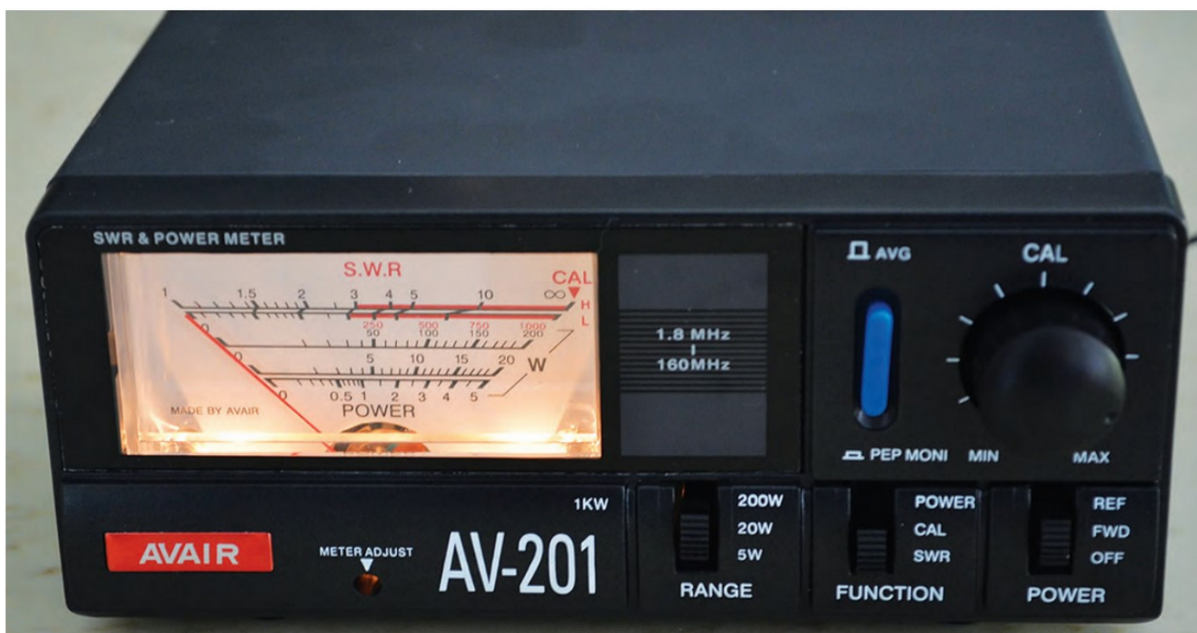
The metal-boxed meter is capable of working in the range 1.8-160MHz.
