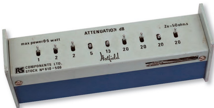
PHOTO 1: Switched attenuator – these can often be found as surplus at rallies and from some of the second hand equipment suppliers. The one shown is good up into the VHF region.
