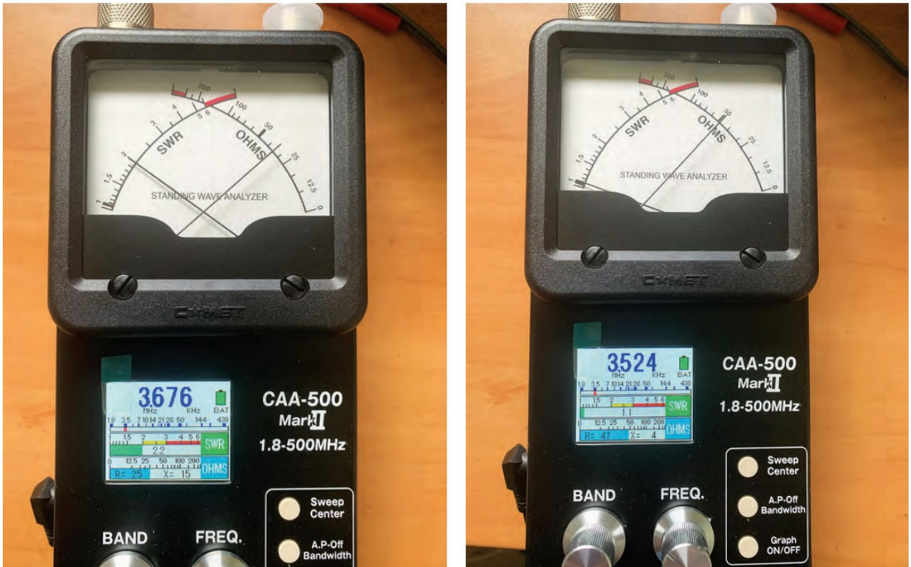
The CAA500 Mark II came in handy for adjusting the reviewer's 80m dipole. The lead image shows the readings in SSB part of the band, with SWR around 2:1, whilst the right image shows the antenna almost resonant on the CW part of the band.
