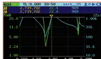
FIGURE 12: Resonance around 1.8MHz.
