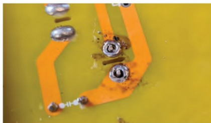
PHOTO 4: The desoldering tube can leave very clean holes and is especially useful when working on double sided boards with plated-through holes.
