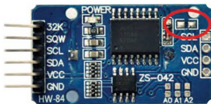
PHOTO 3: The RTC module. I removed the resistor from the pads ringed in red (see text).
