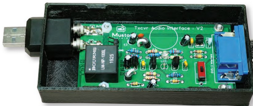
PHOTO 3: Completed board in enclosure. Note how 3.5mm plugs are soldered to the PCB to plug into the USB sound dongle.
