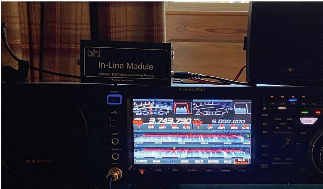
PHOTO 2: The unit in action on top of the author's Yaesu FTDX101MP on 3.743MHz.
