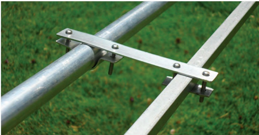
PHOTO 2: The Gamma Match's adjustable strap.
