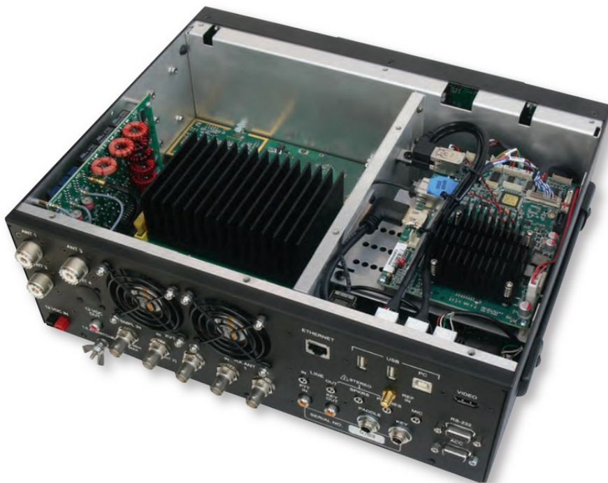
K4 top view with cover removed showing the PA, ATU and single board computer.
