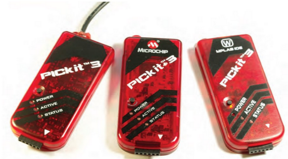
PHOTO 1: Three PicKit-3 programmers. The one in the middle is an original genuine Microchip product. The other two are far-eastern copies, using the same internal controller PIC and firmware, but totally different circuitry with lower levels of protection against overload and mis-connection.
