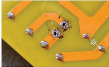
PHOTO 1: A solder sucker often leaves little fillets of solder that cling on to a component leg.
