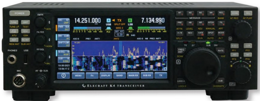
The Elecraft K4 front view is dominated by the display and this is central to the whole operation of the radio. At 7 inches diagonal in size, it is a full colour high-resolution LCD touch screen.
