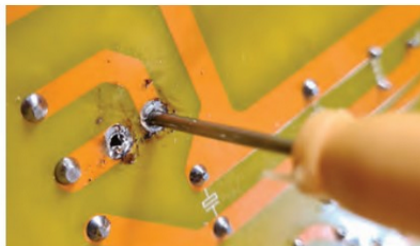
PHOTO 3: Slip the right size tube over the component leg as you heat the joint.
