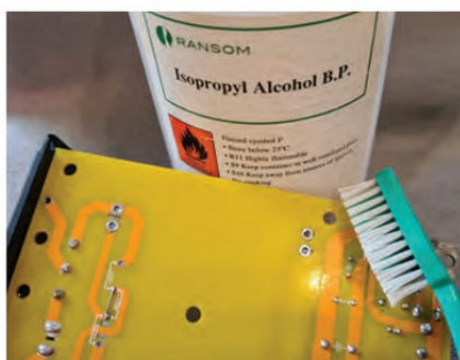
PHOTO 5: A final clean-up with an old toothbrush and some isopropyl alcohol (or meths) and you're good to go.
