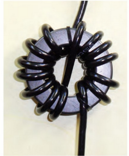
PHOTO 3: Example of a 1:1 choke balun for the HF bands.
