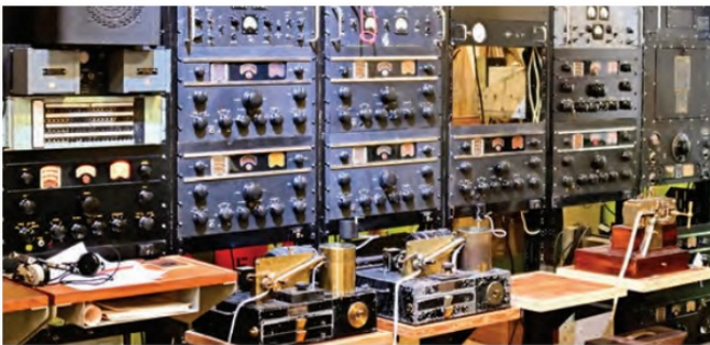
PHOTO 2: Rack of vintage AR88s (with Undulators in front) at The National Museum of Computing.
