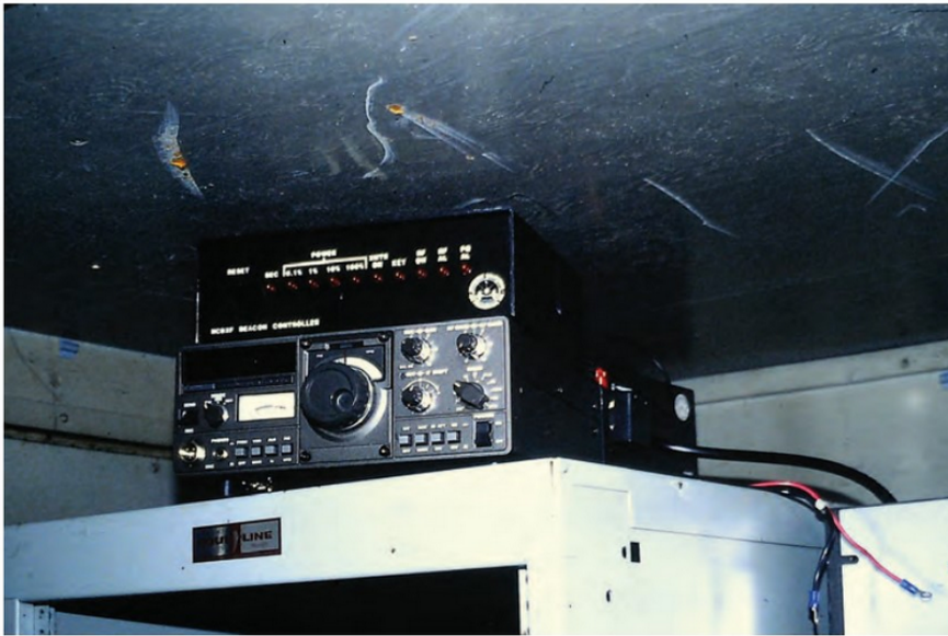
The equipment is a TS-120 plus phasing unit designed by Mike, K6MYC.
