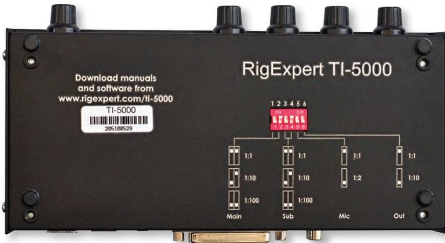
PHOTO 3: DIL gain switches on the underside of the TI-5000.
