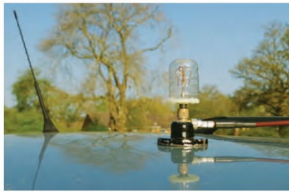
PHOTO 1: 2.4GHz Quadrifilar Helix antenna used for QO-100 uplinks tests using the JT9G-Fast and JT9H-Fast modes.
