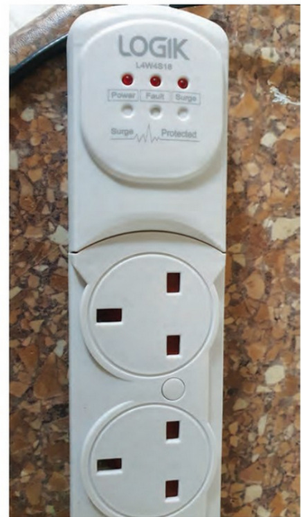
PHOTO 1: The offending 10m-resonant extension lead.
