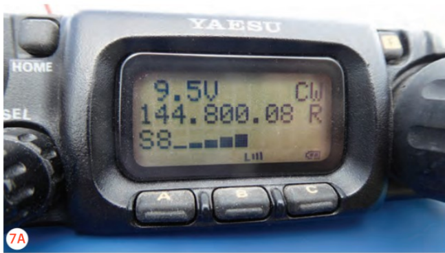
PHOTO 7A-B: On top of Ditching Beacon receiving the Isle of Wight beacon (1296.800MHz) S8 using a dipole on the PE1CMO receive converter and using a FT-817 (tuned to 144.800MHz).
