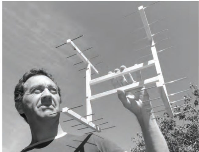
PHOTO 5: As the 1296MHz band wavelengths are a tenth of those on the 144MHz band, the antennas are proportionally smaller.
