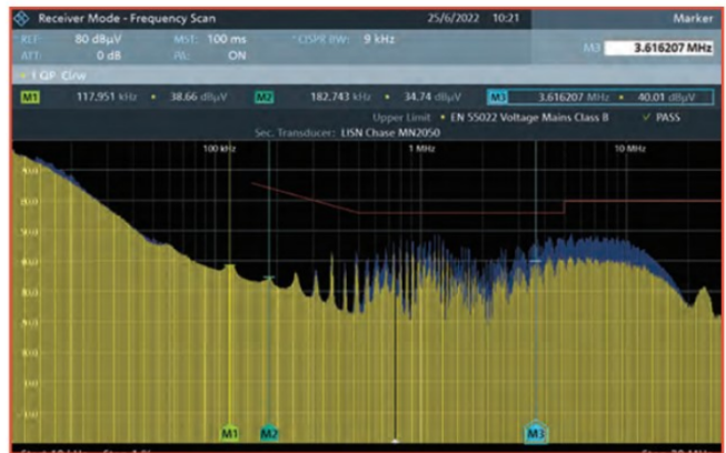
FIGURE 3: Mains conducted emissions from 5V security camera PSU with load grounded via 150Ω (yellow) and DC output conducted emissions (blue).
