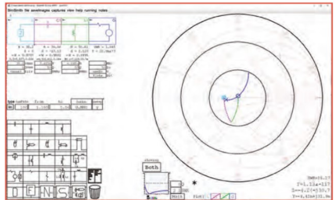
FIGURE 4: L-network solution after invoking the 1:16 transformer on the input.
