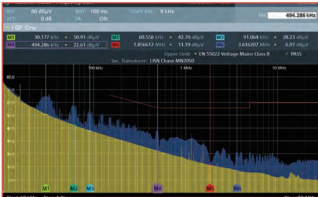
FIGURE 1: Mains conducted emissions from Raspberry Pi PSU (blue) and measuring system noise floor (yellow).
