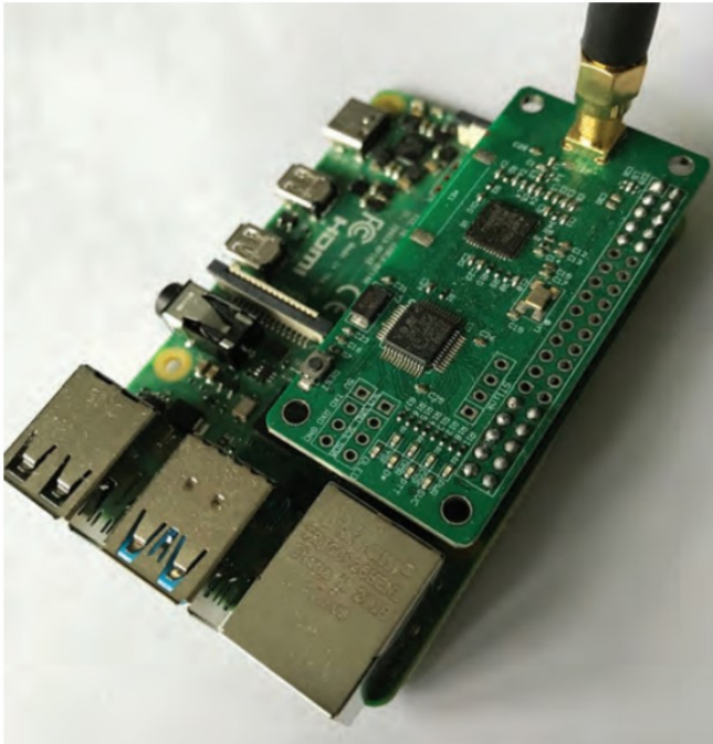
PHOTO 2: The MMDVM Hat simply plugs onto the RPi.
