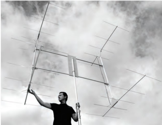
PHOTO 5: As the 1296MHz band wavelengths are a tenth of those on the 144MHz band, the antennas are proportionally smaller.
