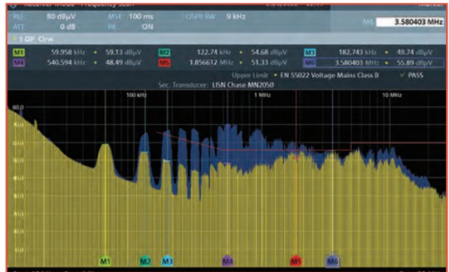
FIGURE 2: Mains conducted emissions from 5V security camera PSU with load floating (yellow) and load grounded via 150Ω (blue).
