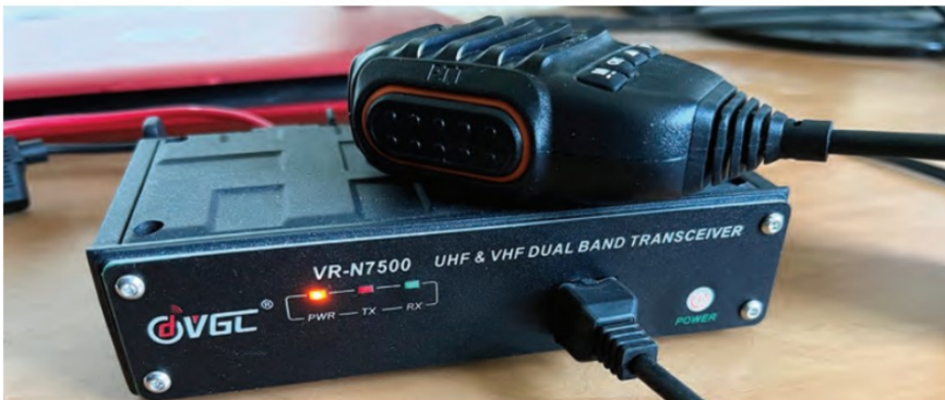
The Vero VR-N7500 does not have a control panel so can be mounted in the boot of your car.
