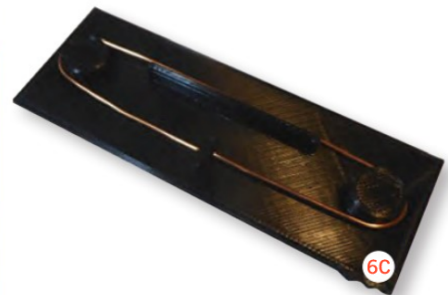
PHOTO 5: As the 1296MHz band wavelengths are a tenth of those on the 144MHz band, the antennas are proportionally smaller.
