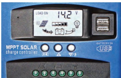
PHOTO 4: An MPPT solar charge controller has the highest efficiency.
