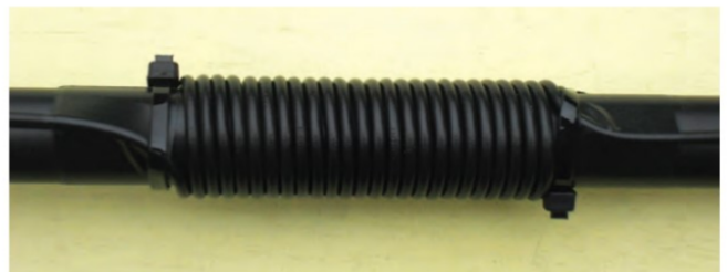
PHOTO 3: An example of one of the 25-turns loading coils used for the antenna.
