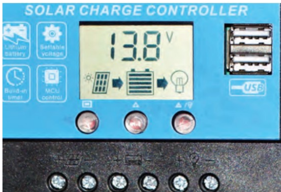
PHOTO 5: PWM charge controllers are cheaper than the MPPT type.
