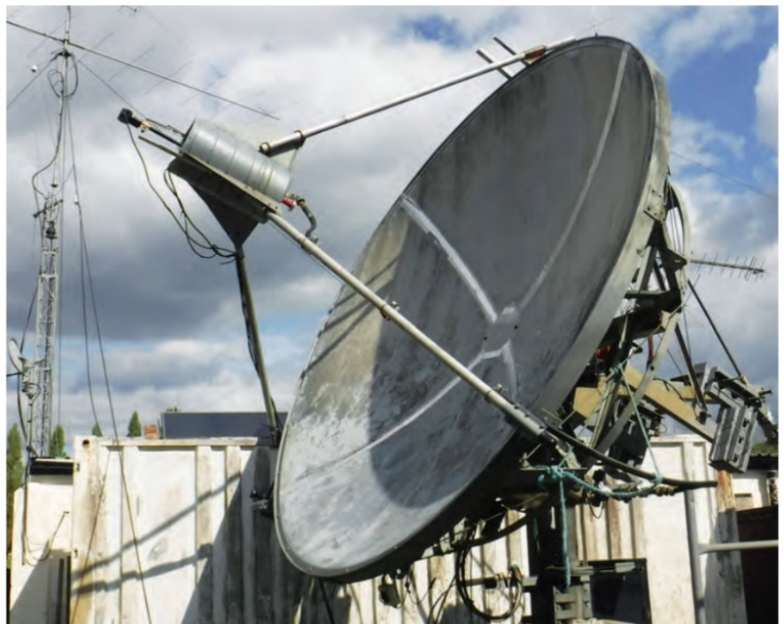
PHOTO 2: The 3.2m dish used by the Flight Refuelling ARS EME Group. Courtesy John, GOAPI.
