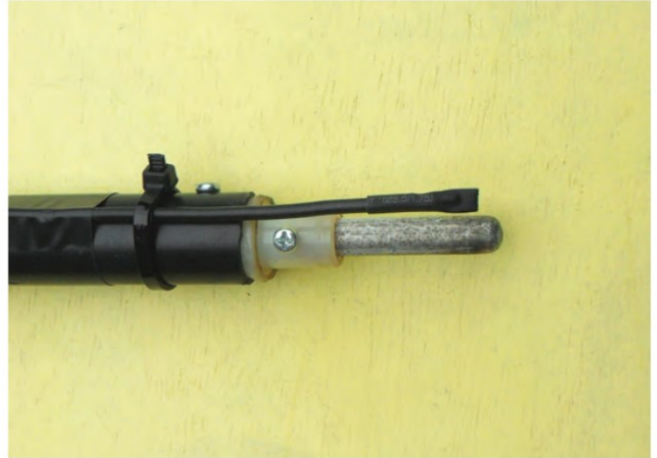
PHOTO 2: An example of one of the tuning rods and its bush mount used for the antenna.
