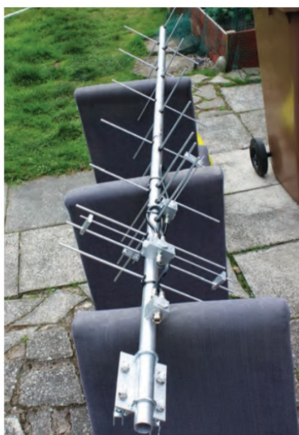
70cm Yagi after construction was completed.
