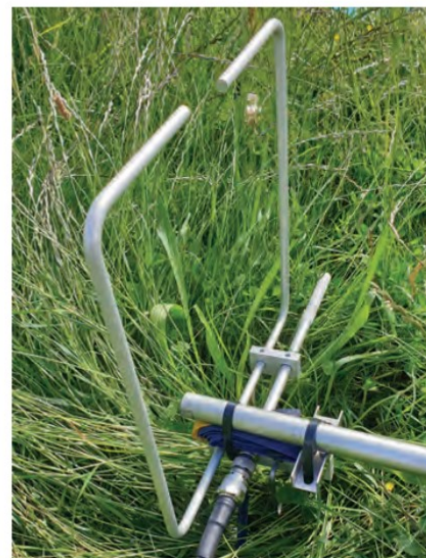
The Sharman Halo antenna close up. It comes with a proper mast clamp, but here I improvised with cable ties to fix it to my narrow fibreglass mast.
