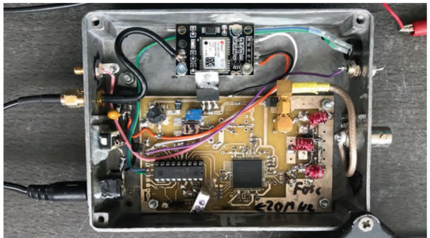
PHOTO 1: 144MHz chirp generator based around an AD9852 DDS module and PIC controller. A GNSS receiver module, seen at the top, supplies timing information to ensure a start time for the chirp controlled to within less than a microsecond of UTC.
