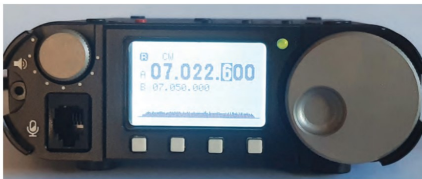
PHOTO 1: The Xiegu G106 front panel with liquid crystal display, similar to the GM1 version.
