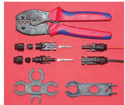
PHOTO 2: MC4 components. (Top) crimping tool; (middle) connectors; (bottom) assembly/disassembly tools.
