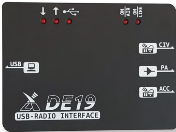
PHOTO 3: The DE-19 USB to radio interface uses a USB C connector towards the PC for CAT control and audio.
