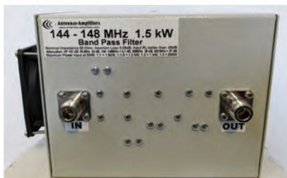
The front of the bandpass filter, displaying the N-Type connectors for the input and output.
