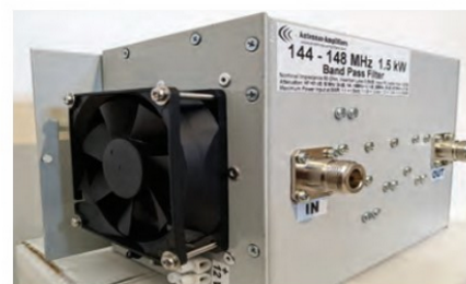
The left-hand side has a PC-style 12V exhaust fan to help with heat dissipation at high power levels.
