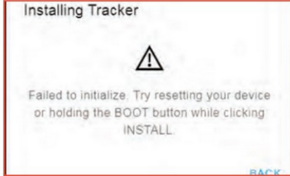
In case of an error, GPIO0 must be connected to GND before programming the TTGO.
