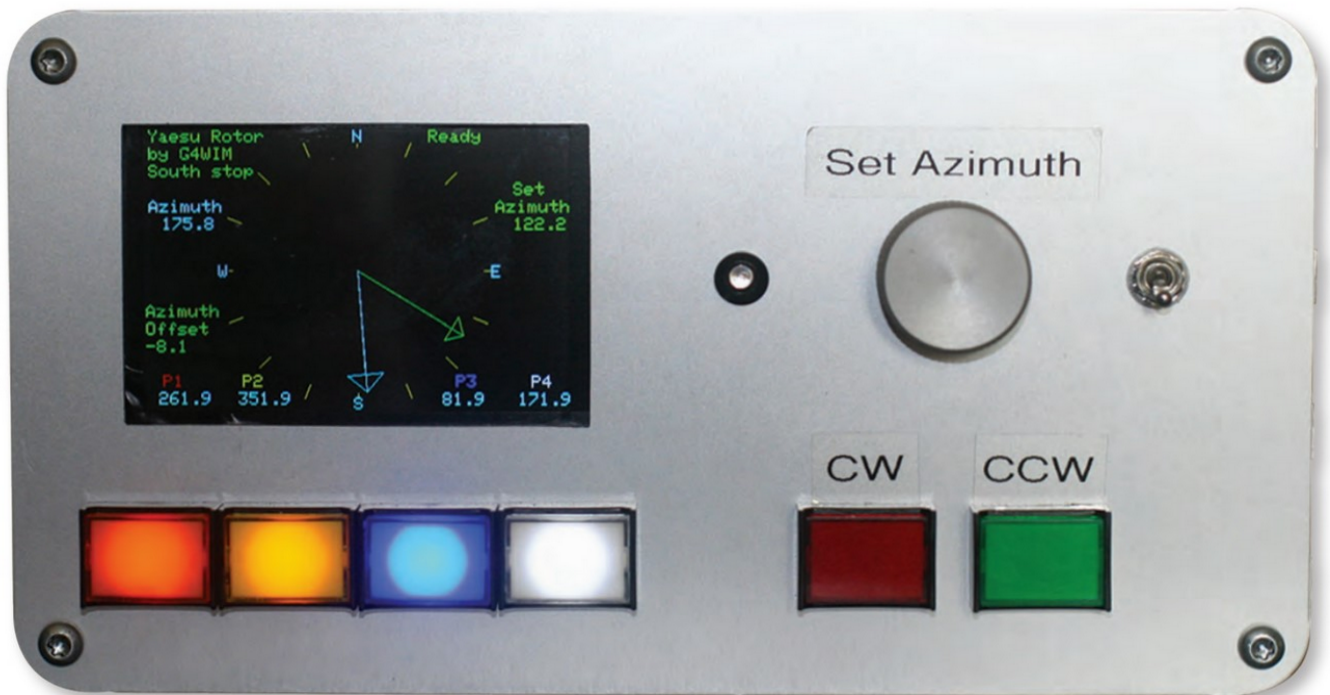
Photo 1: Front panel of the rotator controller, 4 preset buttons, CW & CCW and Azimuth control.
