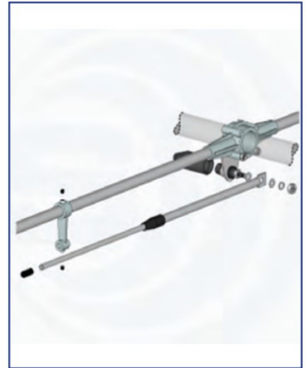
FIGURE 3: The Gamma Match of the Syro 27-4.
