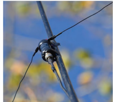
Dipole centre mounted on a pole.
