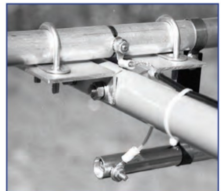
PHOTO 3: Connecting the Coax to the antenna (credit QST Magazine).
