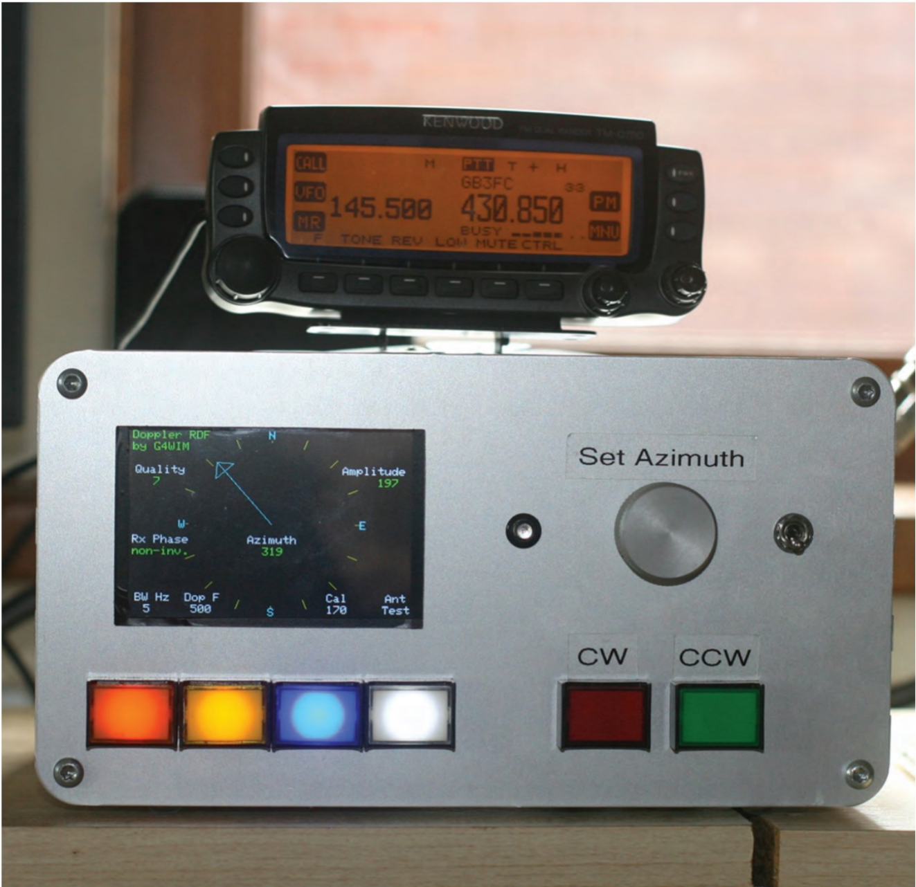
PHOTO 2: The RDF screen displays the Azimuth Data.
