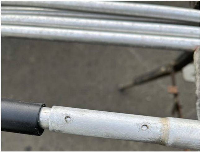
PHOTO 5: Always clean the tube joints on the elements.
