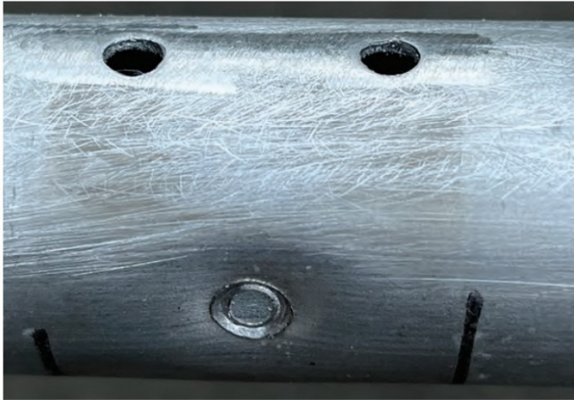
PHOTO 4: Always remove the burs from the tubes.
