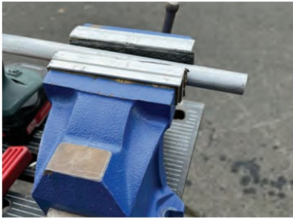
PHOTO 8: Hold the work with a good vice.
