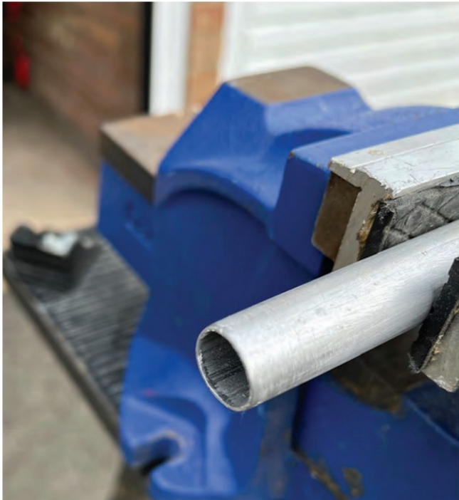
PHOTO 6: Always tidy the sharp burs from the ends of the tubes.
