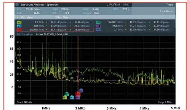
FIGURE 1: Substation RF interference measurement 50kHz - 5MHz.
