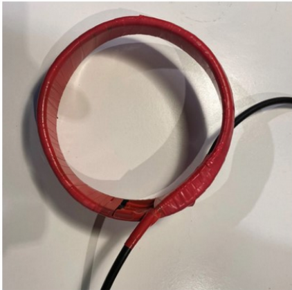
PICTURE 2: The completed choke, with five turns of RG-58 wrapped initially around a 110mm diameter soil pipe to help construct the choke.
