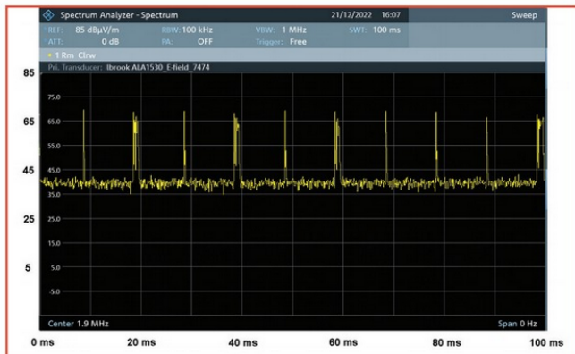
FIGURE 2: Substation RF interference measurement zero span mode, 100ms span.
