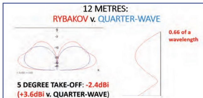
FIGURE 3: Rybakov versus quarter-wave antenna on the 12m band.
