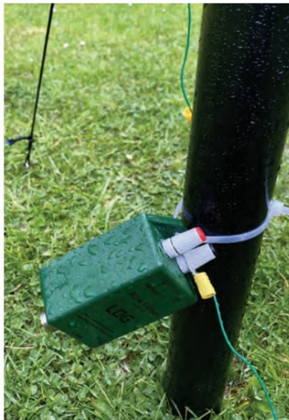
PHOTO 1: 4:1 UNUN attached to fibreglass pole
