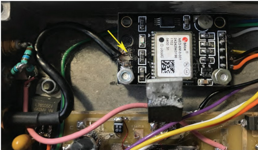
PHOTO 2: the soldering of the inner of the coax connection had failed at the point marked. When tested with a meter probe it was pushed onto the PCB pad showing, apparently, no fault.
