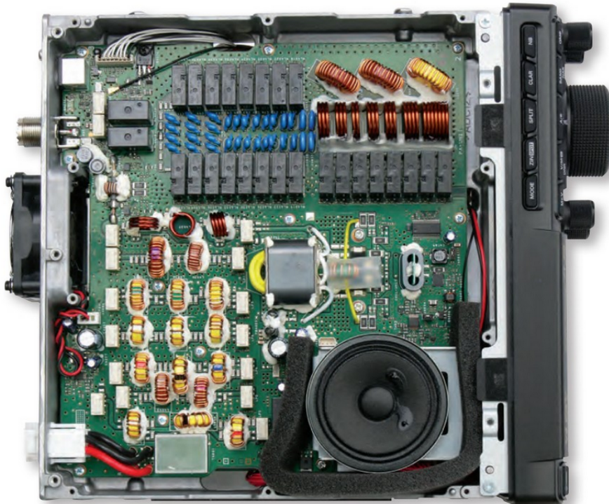
PHOTO 4: Top view with covers removed showing Tx, PA and ATU.
