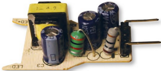
PHOTO 2: LED driver in a GU10 lamp, component side.
