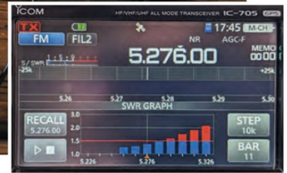
PHOTO 5: In use matching an end-fed half-wave antenna.
