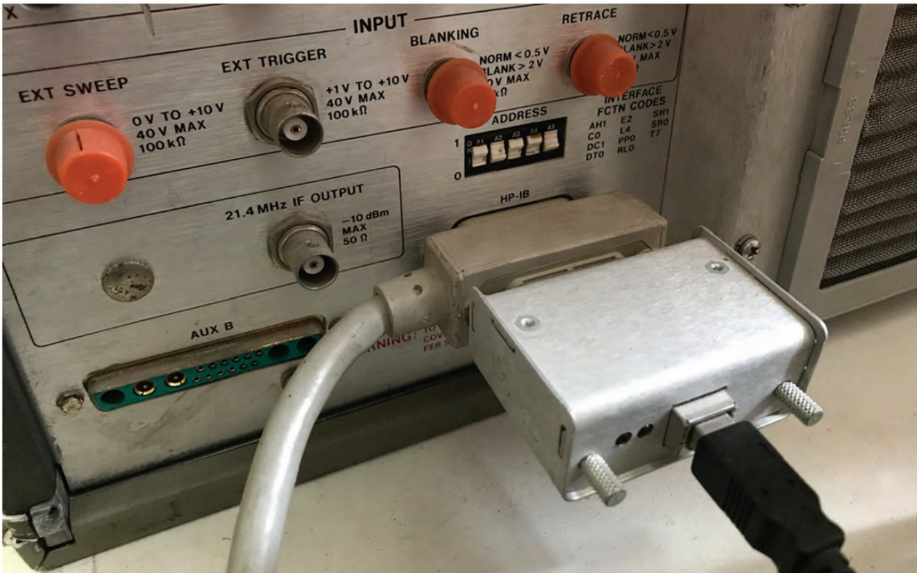
PHOTO 1: HP-IB connector with Prologix interface unit. The switches for setting the equipment address are visible just above the connector.
