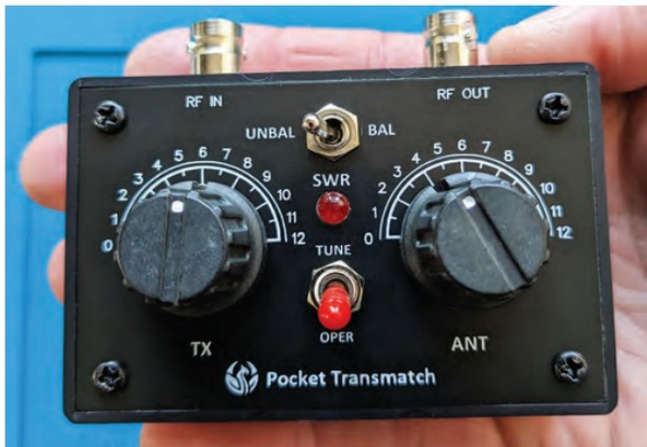
PHOTO 1: The finished ATU.
