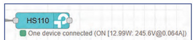
FIGURE 3: The Kasa plug node showing the connect message.
