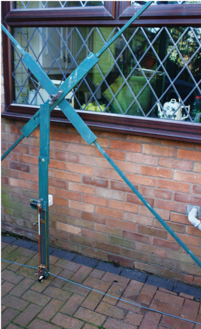
FIGURE 3: A view of the tuner mounted on the wooden support frame of the antenna.
