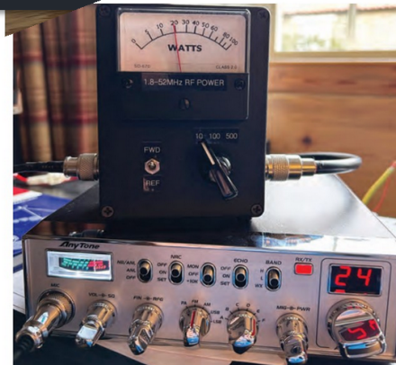
PHOTO 4: Measuring the power output.
