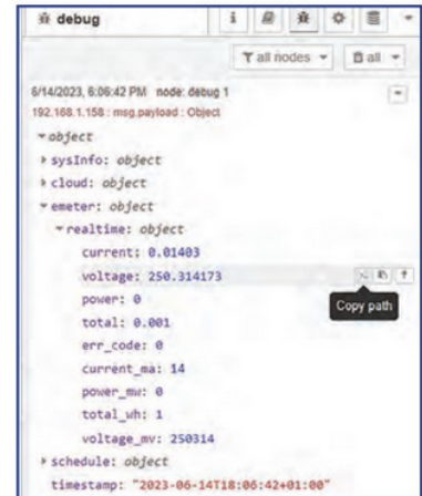
FIGURE 5: Expanded JSON message from the Kasa plug.
