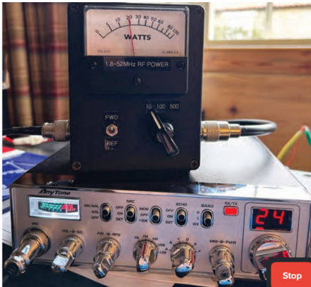
PHOTO 4: Measuring the power output.
