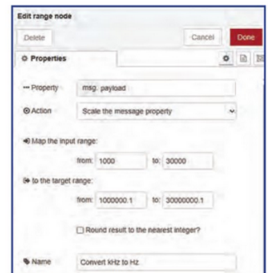
FIGURE 7: Configuring the Range flow to scale from kHz to Hz.
