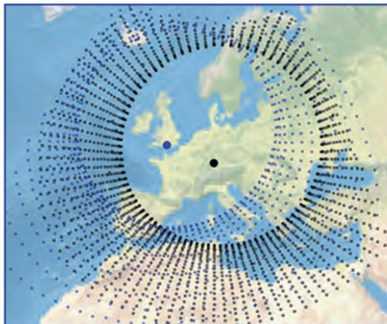
FIGURE 7: Map showing the location of the transmitter at DF4UE (black) and receiver at G3ZIL (blue) together with the landing spots of rays from PyLap 3D ray tracing for 0000UTC on 26 June 2023. It is likely the propagation path was via sidescatter from the regions of greatest landing points overlap.
