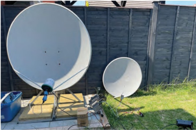
FIGURE 8: QO-100 testing with a 1.2m dish for Tx, and a smaller dish for Rx.
