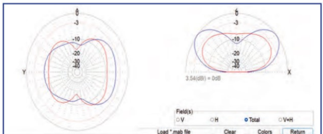
FIGURE 8: On 10m, my adapted version (blue curve) has a peak gain once again at the end opposite the feed point, measuring -0.8dBi. Current here is vertical in direction and is very favourable compared with a quarter-wave or half-wave vertical antenna. Overall coverage in azimuth is competitive compared with the conventional voltage-fed Half-Square antenna (red curve).
