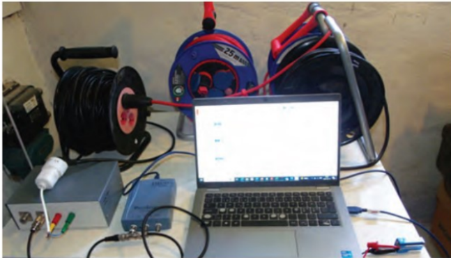
FIGURE 4: Measuring 4 x 25m lengths of mains extension leads using TDR.
