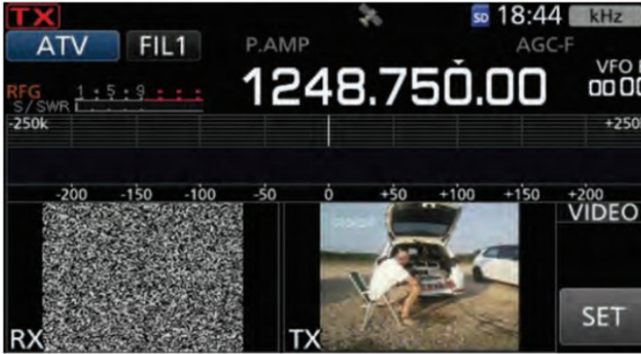
FIGURE 4: A screenshot showing both transmit and received pictures.
