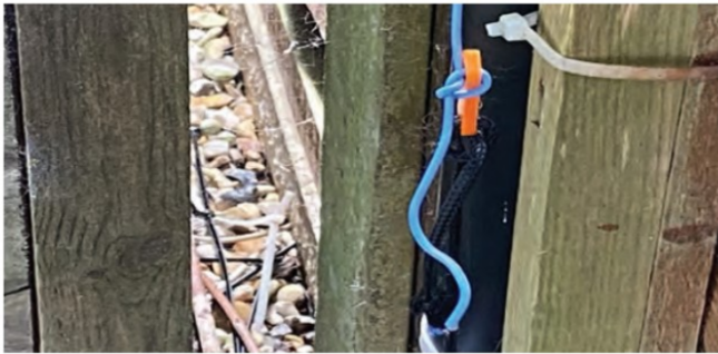
FIGURE 4: The wire opposite the fed-end with it terminated 30cm above ground level.
