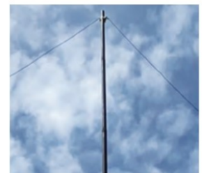
FIGURE 3: The apex of the inverted-V aspect of the antenna, at 8m above ground level.
