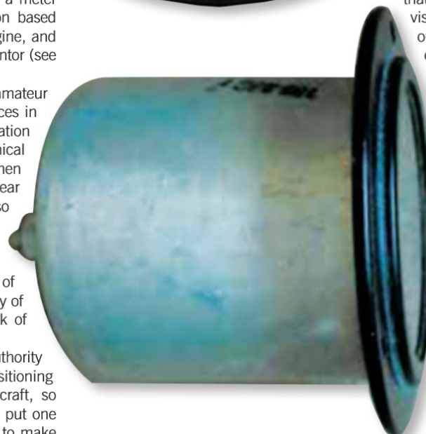
FIGURE 1: An aircraft Hobbs meter: above front view and below side view.
