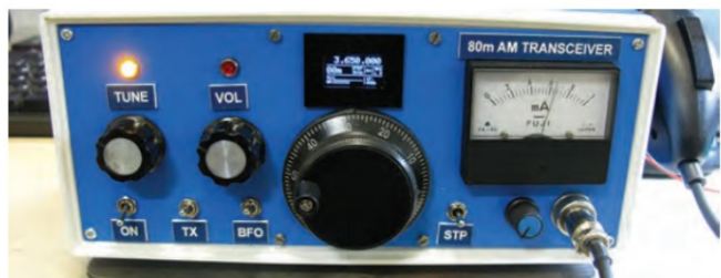
FIGURE 9: G4AQB's homebrew 'class E' transceiver.
