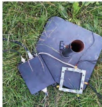
FIGURE 2: The remote ATU sitting on a parasol stand along with a homebrew radial plate.
