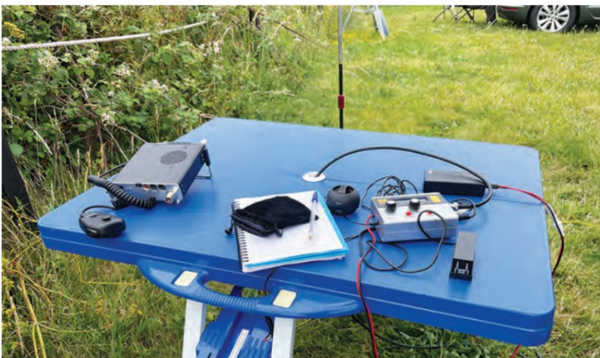
PHOTO 7: A QCX transceiver in use with the antenna on the 20m band.
