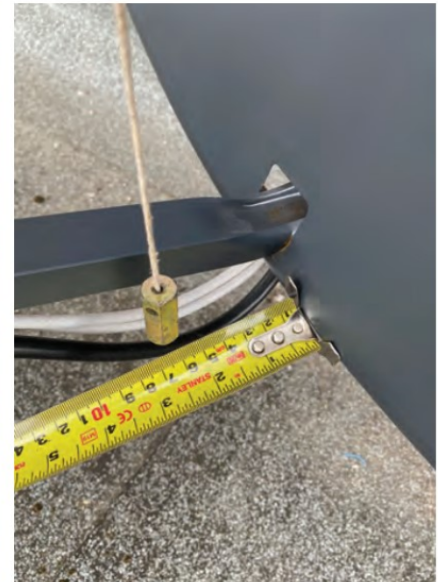
FIGURE 4: Measuring the elevation angle.
