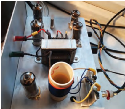
FIGURE 10: G4JQT's homebrew 5MHz copy of the Codar AT5.
