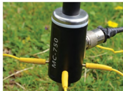
PHOTO 2: The feedpoint installed on top of the ground spike.
