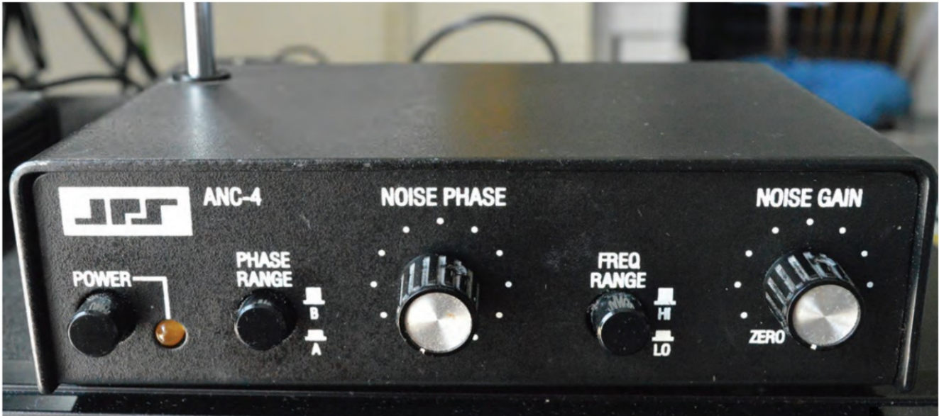
FIGURE 2: The ANC4 noise canceller in use (the screw-in telescopic whip is shown at the top far left).
