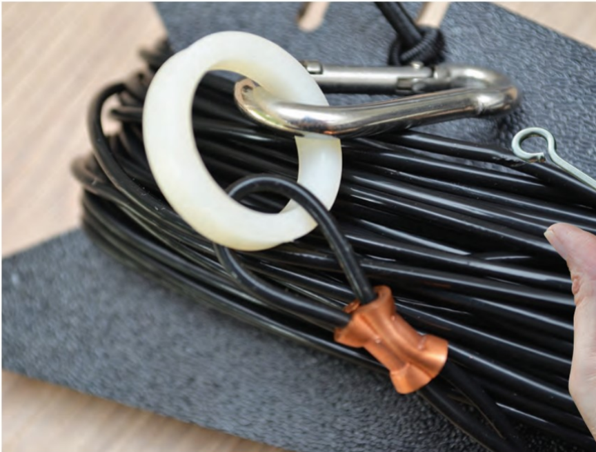
FIGURE 3: One of the dipole arms folded for transport, showing the end fixings.
