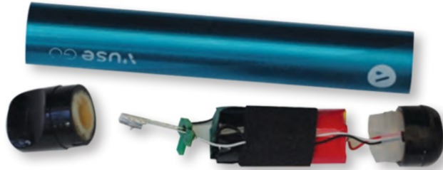
FIGURE 5: The typical innards of a disposable vape, showing the heating element, battery and bottom cap containing the sensor. The top cap/mouthpiece has also been separated.
