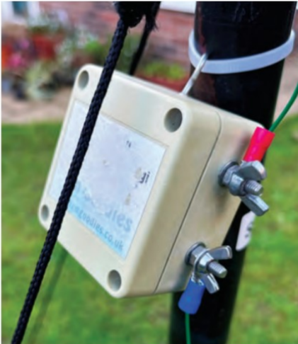
FIGURE 4: The 9:1 UNUN and elements.
