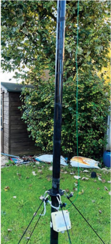
FIGURE 5: Upper element and guyed pole.
