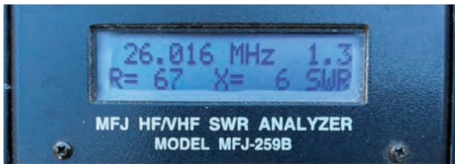
FIGURE 6: VSWR reading before any adjustments, showing the best VSWR below 10m.
