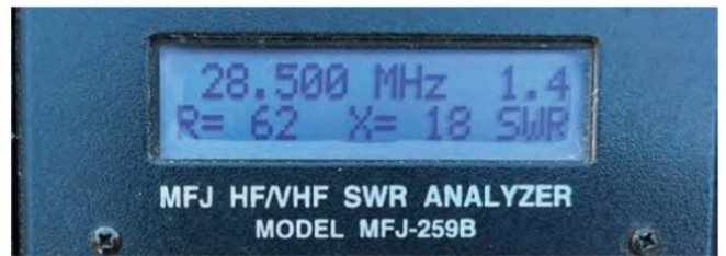
FIGURE 7: VSWR reading for 10m after shortening the antenna.
