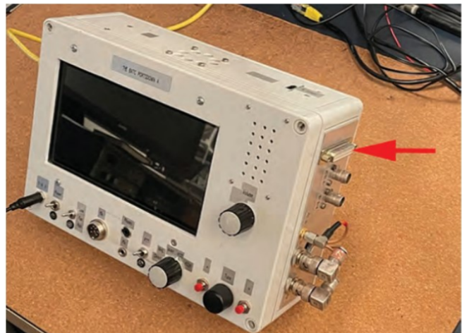
FIGURE 7: The Portsdown system in a plastic enclosure with the standard interface indicated by the red arrow.
