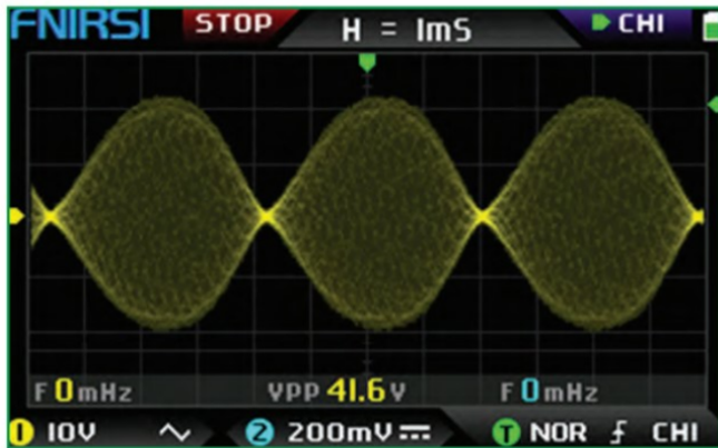
FIGURE 3: A two-tone SSB test at 144MHz using a Yaesu FT-817.
