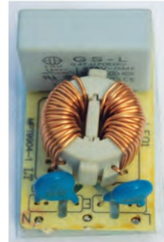
PHOTO 3: A mains RFI filter PCB.
