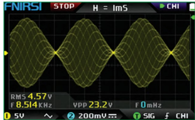
FIGURE 4: A two-tone SSB test at 1.81MHz using a Yaesu FT-710.
