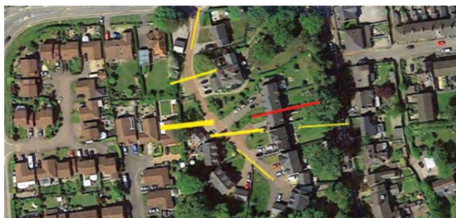
FIGURE 8: An initial search. The yellow lines indicate the directions to the source of interference, with the thicker lines indicating increased signal strength. My 80m dipole is shown in red.
