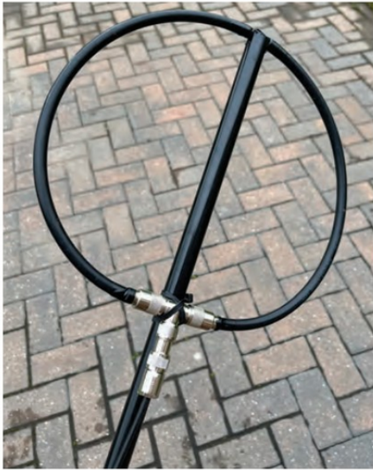
FIGURE 4: The original loop antenna.
