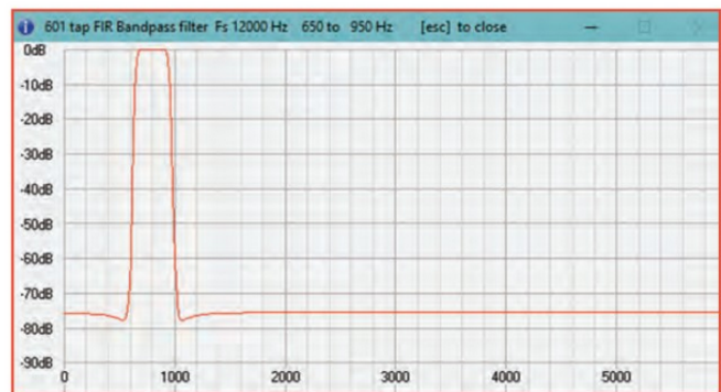
FIGURE 12: The calculated frequency response of the band-pass digital filter with a 'Hamming window' applied in the Fourier transform, with 601 coefficients.
