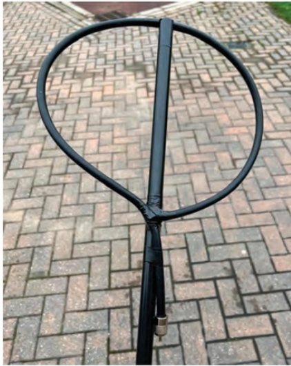
FIGURE 6: The finished loop Mk2.
