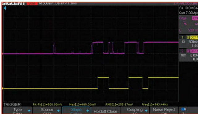
FIGURE 1: Oscilloscope traces showing the voltage before de-bouncing (magenta trace), and after de-bouncing (yellow trace).
