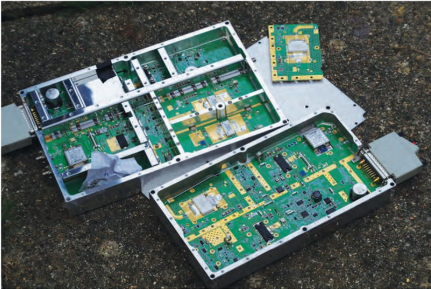
FIGURE 2: Surplus modules from the mobile-phone market. These are worth dismantling to find RF devices for power amplifiers.
