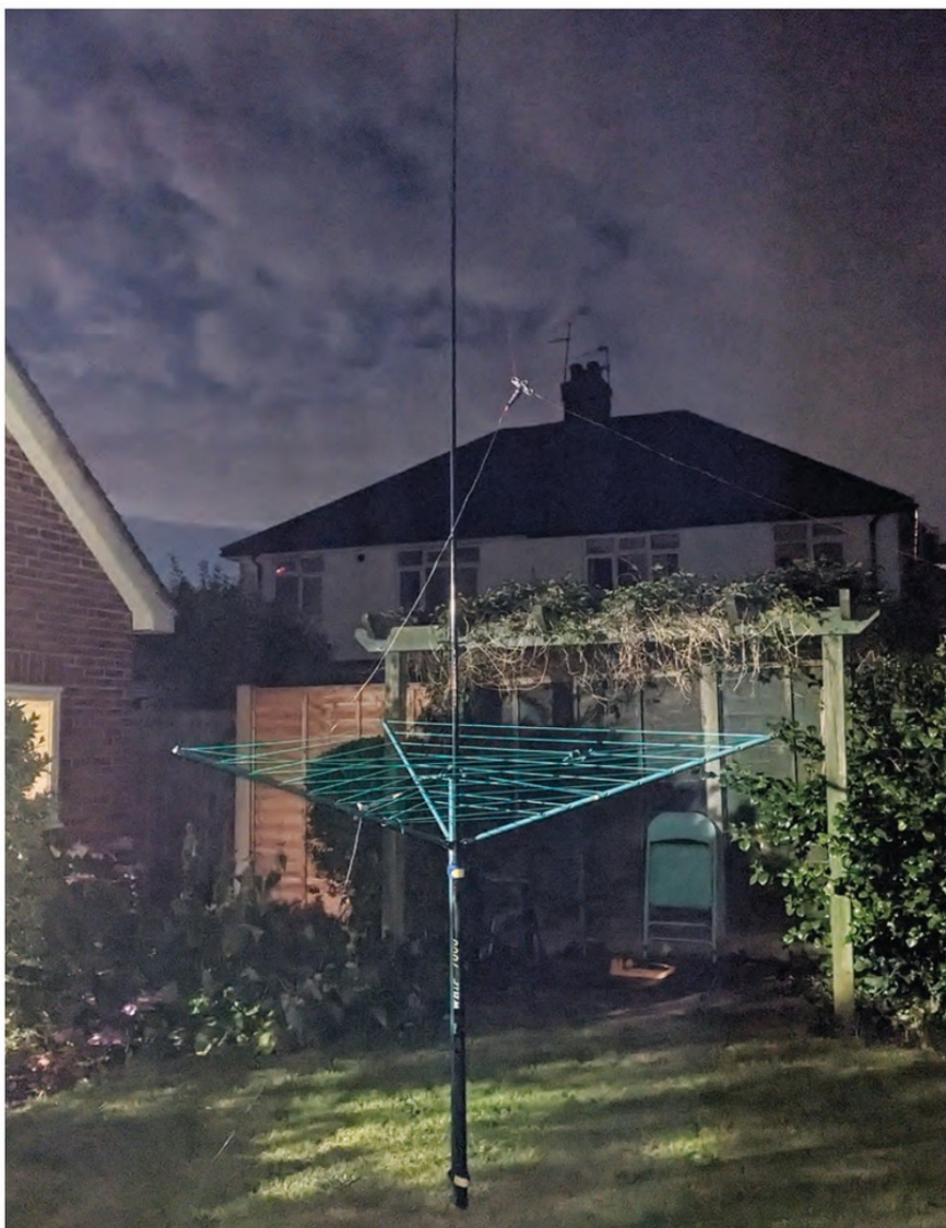
FIGURE 1: The 6m dipole erected in my small garden.
