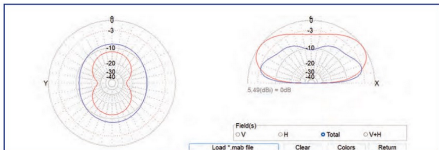
FIGURE 6: A comparison between the horizontally- and vertically-polarised delta loops using the 7m pole as support; red is horizontal and blue is vertical.
