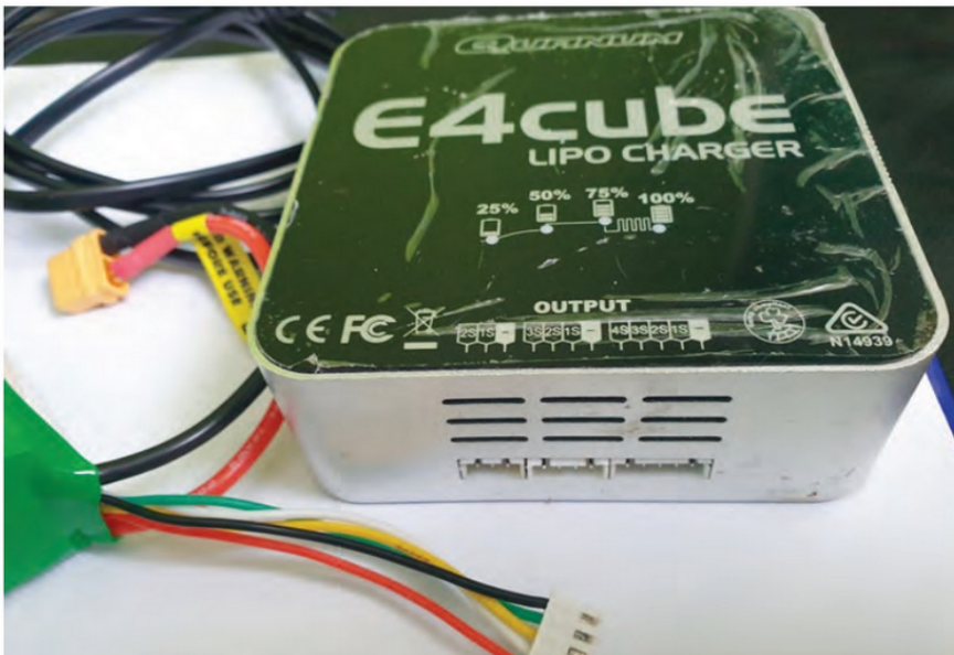
FIGURE 3: The LiPo battery charger.
