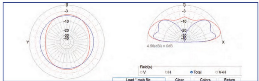
FIGURE 9: A comparison between the vertically-polarised delta and the half-wave vertical antenna using the 10m pole; red is the loop and blue is the vertical antenna.
