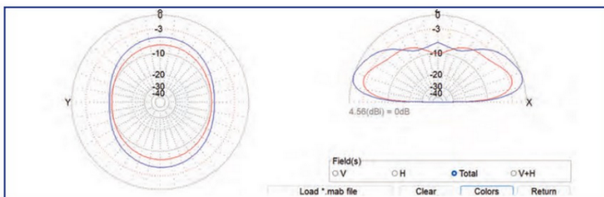
FIGURE 4: A comparison of the azimuth and elevation far-field plots when using 7m (red) and 10m (blue) support poles for the vertically-polarised delta loop.
