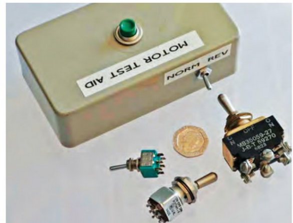
FIGURE 2: A selection of centre-off control switches of various sizes and vintages.
