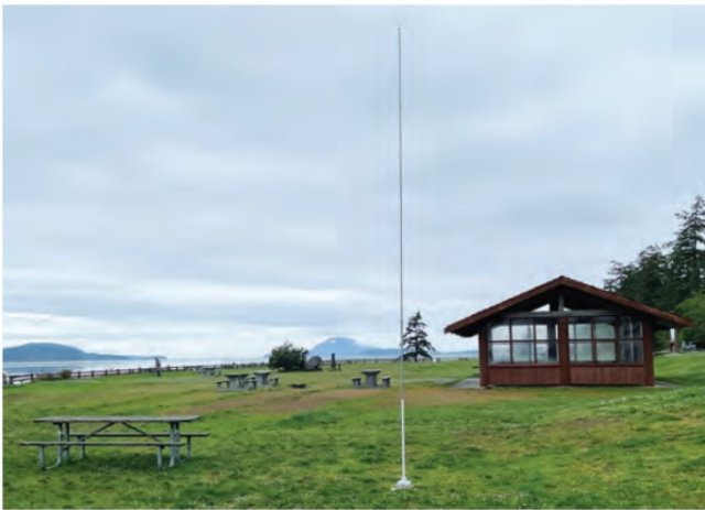
FIGURE 5: A Porcupine with a 40m home-made telescopic whip, showing the extra piece of PVC pipe for additional support.
