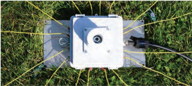
FIGURE 4: The radial field without a vertical element fitted.
