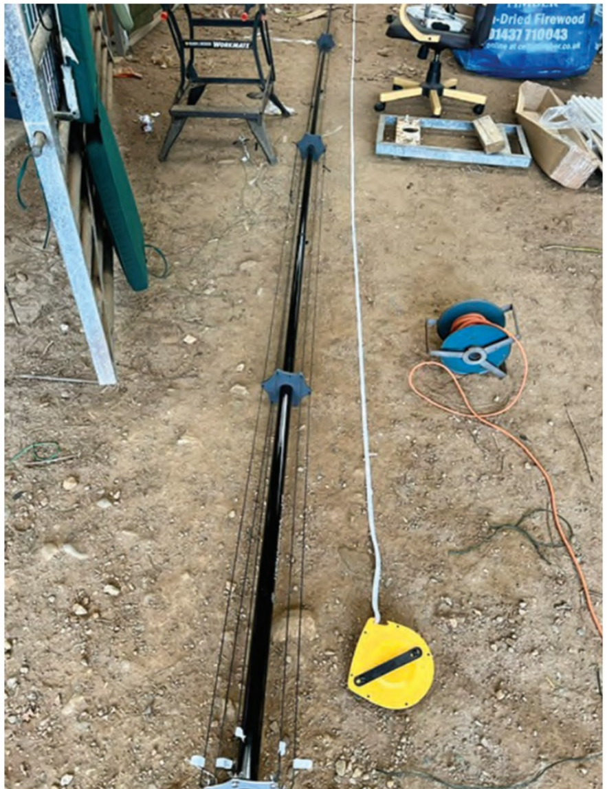
FIGURE 1: The antenna being assembled on the ground.
