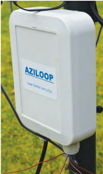
FIGURE 2: The DF-72 loop control unit (LCU).
