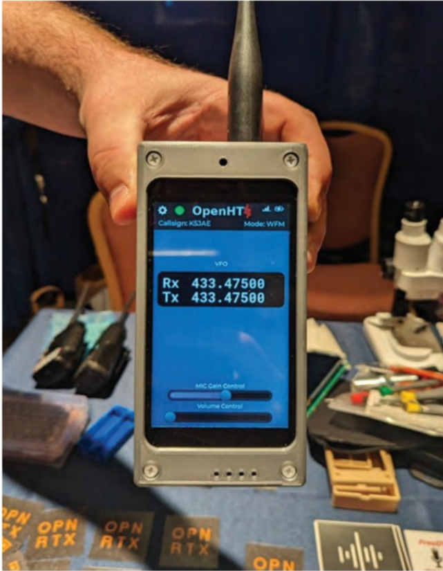
FIGURE 1: OpenHT, an open-source SDR-based handheld transceiver.
