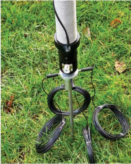
FIGURE 3: The base of the antenna secured in the ground by the spike before deploying the radials.
