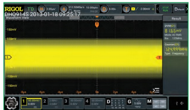
FIGURE 17: A 125MHz waveform with aliases.
