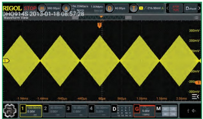
FIGURE 14: A 1MHz sine wave, amplitude modulated by a 1kHz triangular wave at 100%.
