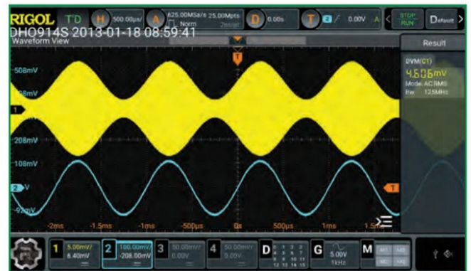
FIGURE 19: The same AM waveform as in Figure 18, with no aliases.
