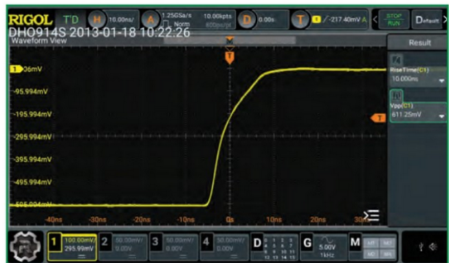
FIGURE 5: The probe rise time in the 1:1 position is 10ns (provided by Telonic).
