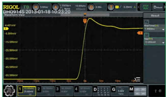
FIGURE 6: The probe rise time in the 10:1 position is 1.85ns (provided by Telonic).
