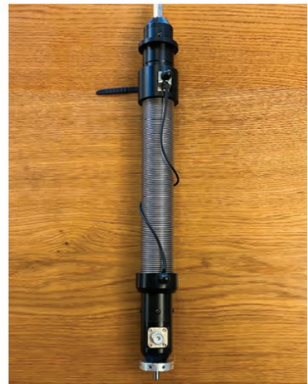
FIGURE 6: The coil assembly showing the collar right at the top.
