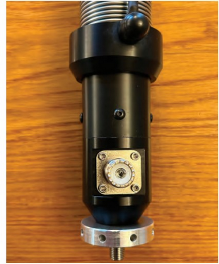
FIGURE 5: Power from the transmitter is delivered via an SO239 connector.
