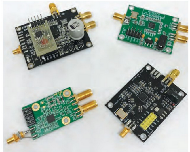
FIGURE 1: A collection of PLL synthesizer modules to be found from many online sellers. Bottom right is the ADF4351 device for 35MHz to 4.4GHz. Then going anti-clockwise, the MAX2870 is broadly similar but covers the frequency coverage from 23MHz to 6GHz. Top left is the 'deluxe' ADF5355 that can generate frequencies in the range 54MHz to 13.6GHz at tiny frequency steps thanks to its double fractional-N architecture. Finally, at bottom left is another ADF4351 module, supplied by SV1AFN, that has an improved board layout for reduced phase noise and spurs, but does need an external voltage regulator.
