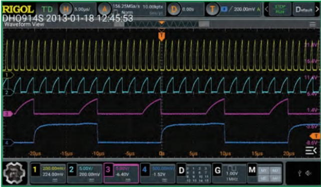
FIGURE 11: The waveforms of a divider chain displayed simultaneously.
