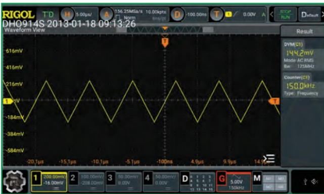
FIGURE 13: A triangular wave generated by the AFG.
