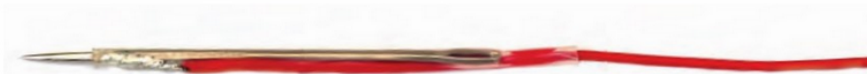
FIGURE 3: Test probe for working on the tiny tracks and pins of SMD printed-circuit boards. This is also useful for probing fuse slots to check which switched circuits they are on.
