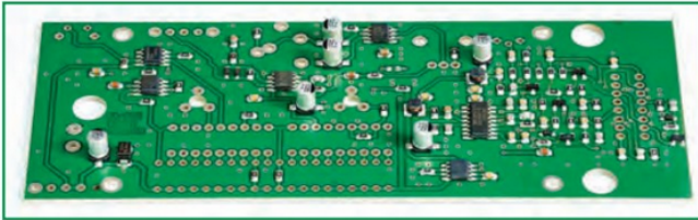
FIGURE 4: The SMD parts come pre-installed.
