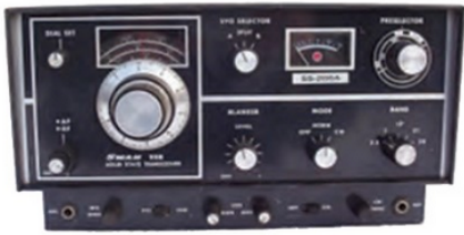
FIGURE 5: The first all-solid-state transceiver: Swan SS-200A, 1973.
