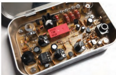
FIGURE 2: The FOXX-3 transmitter, housed in an Altoids tin.
