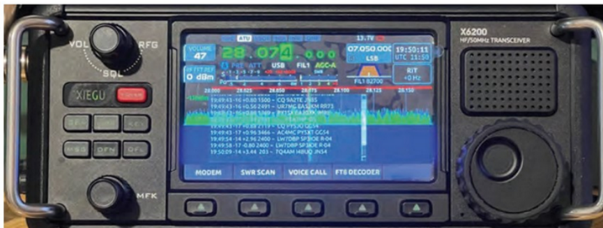
FIGURE 5: The transceiver has a built-in FT8 decoder.
