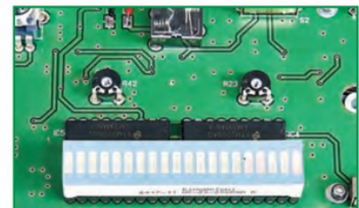
FIGURE 6: R23 and R42 must be adjusted.
