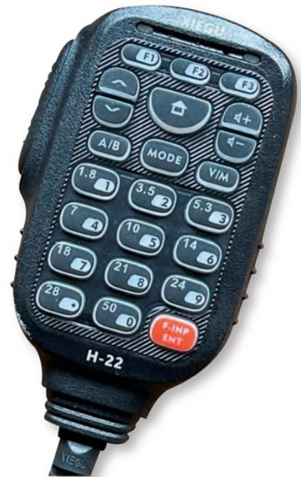
FIGURE 6: The supplied hand microphone with its five buttons for selecting the band and mode.
