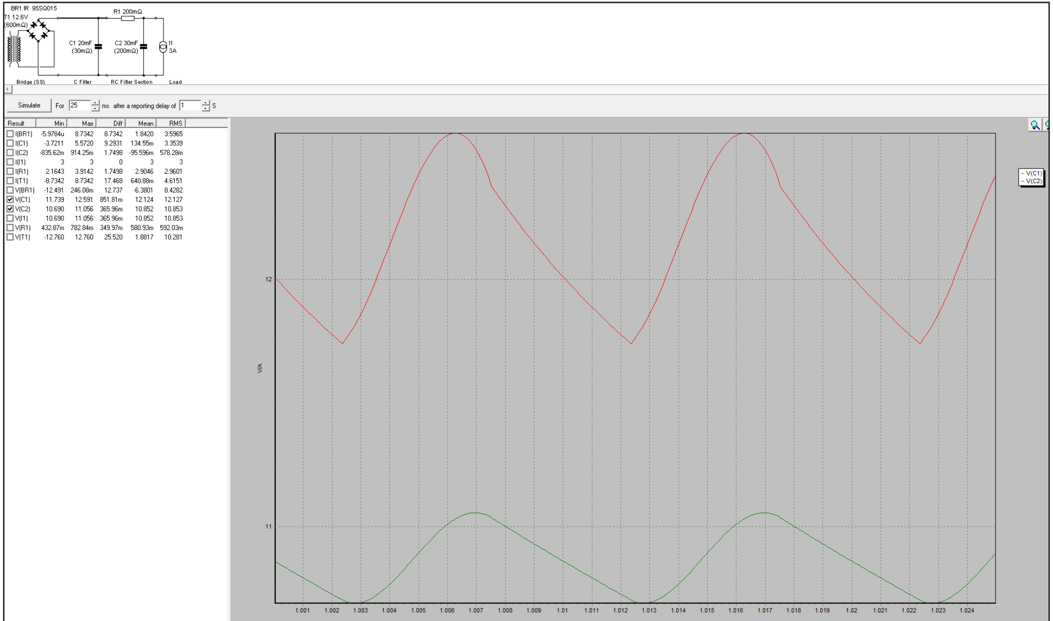
FIGURE 17: The effect of one additional RC network post rectification.
