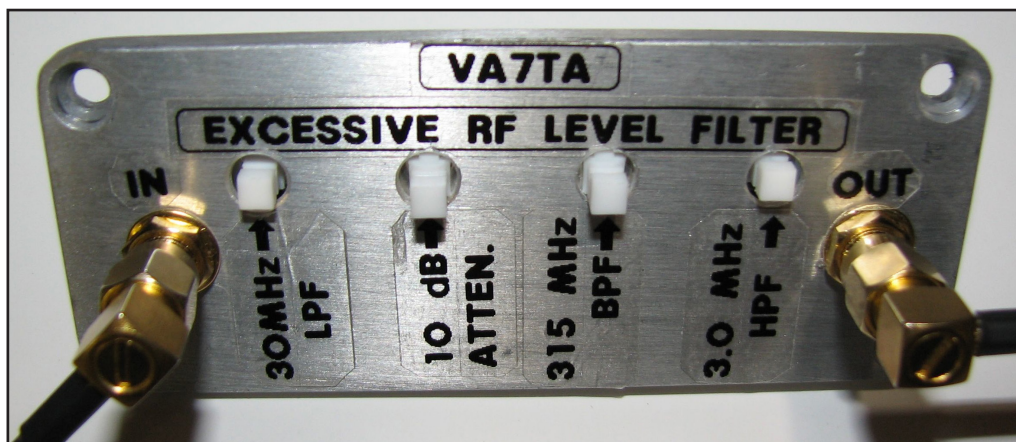
FIGURE 15: The front panel labelled with transparent label tape.
