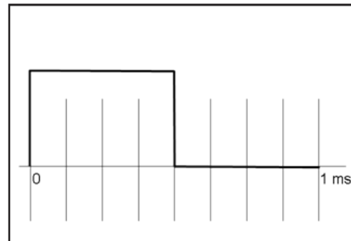
FIGURE 1: A 1kHz square-wave voltage pulse.
