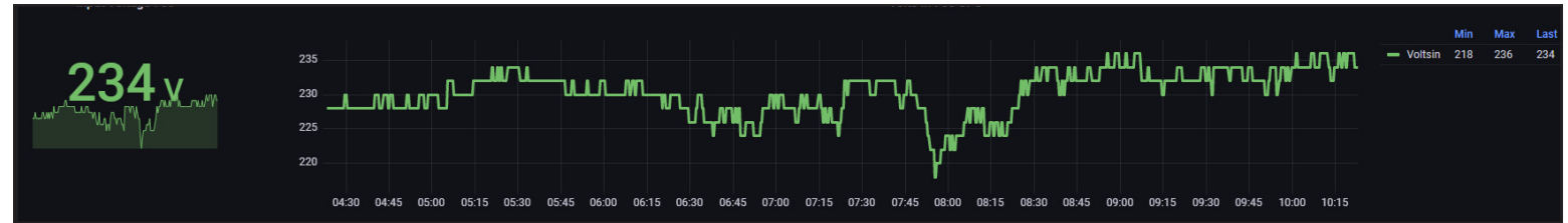
FIGURE 9: The variation of the mains voltage as observed in late December 2022.
