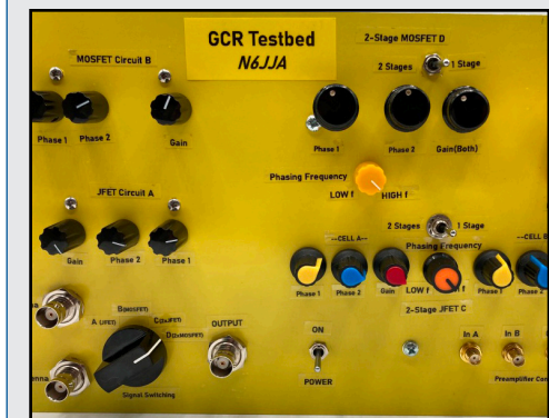
COVER IMAGE 3: Building and testing antenna noise cancellers
