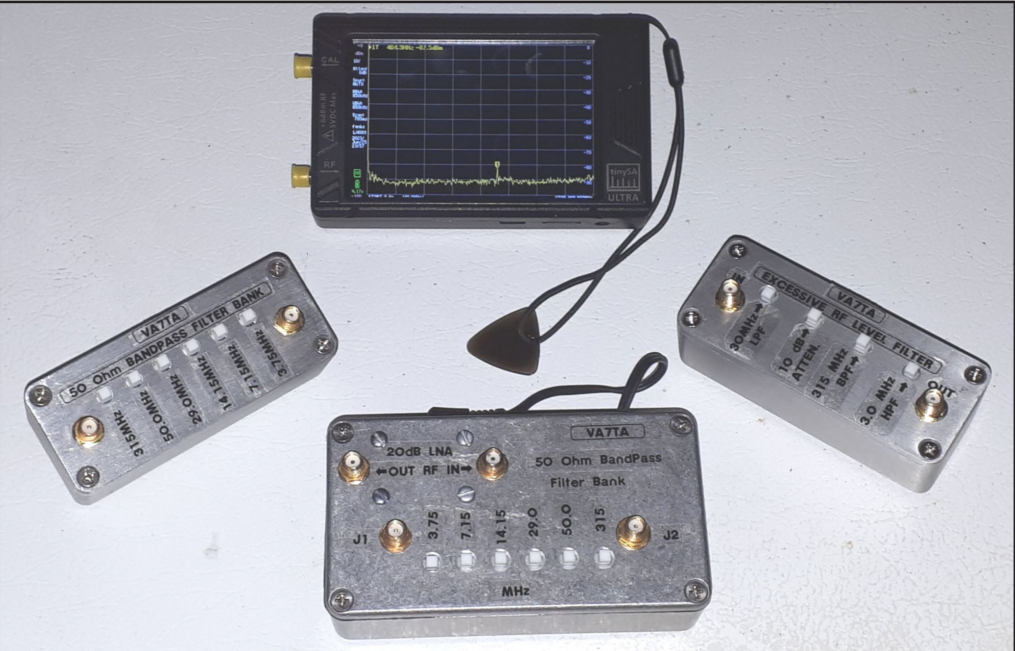
FIGURE 1: My TinySA Ultra handheld spectrum analyzer (top) and three overload-protection filter alternatives: passive high or low pass, band pass, and with or without an LNA for a sensitivity boost.
