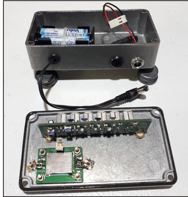
FIGURE 10: The protection filter and 5-600MHz 20dB LNA, purchased online from AliExpress, installed on a Hammond 1590B enclosure lid. The 4 AAA cells and the plug/jack switch assembly is also shown.
