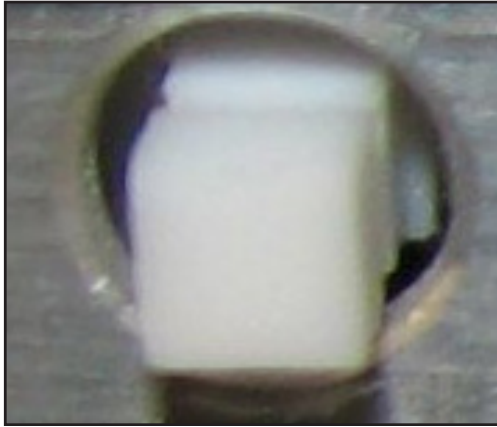
FIGURE 17: A close-up view of a switch-plunger front-panel hole with chamfered edges, taken with a low-power microscope.
