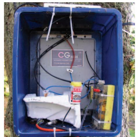
PHOTO 5: The ATU in its tree-mounted box with the lid removed. The aerial relay is inside the pepper carton.
