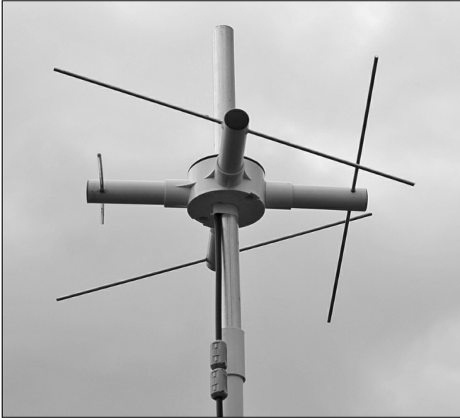
Fig 3: A Lindenblad type antenna using parasitic elements designed by Anthony Monteiro AA2TX a useful omni for the 70cm band
