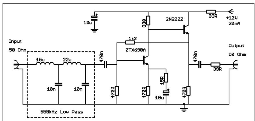
Fig 10.8: 20dB preamplifier
