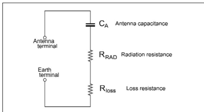
**Fig 10.34: Equivalent circuit of vertical antenna**
