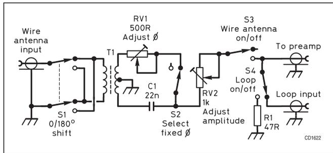
**Fig 10.55:** G3GRO noise canceller. RV1 and RV2 are linear cermet or carbon. T1 is 3 x 18 turns trifilar wound on a ferrite toroid (13.25mm dia. 3C85 ferrite, Amidon FT-50-43 or similar)
