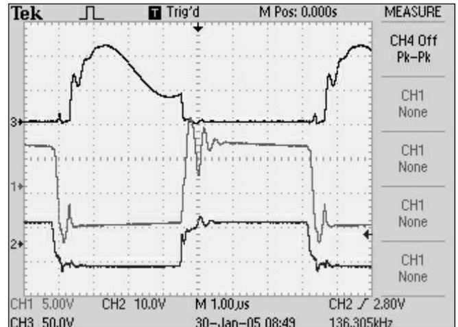
**Fig 10.12: Class D waveforms. Upper trace, drain voltage; middle trace, drain current; lower trace, gate drive voltage**
