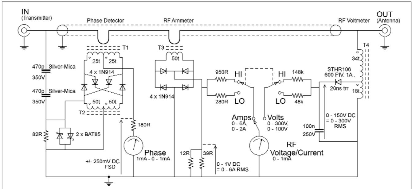
**Fig 10.61: LF Tuning meter circuit.** T1: Primary is RG58 coax passing through core, secondary 2 x 25t bifilar 0.3mm enamelled copper. T2: 2 x 50t bifilar 0.25mm enamelled copper. T3: Primary is RG58 coax passing through core, secondary 50t 0.5mm enamelled copper (see text for details of transformer construction)
