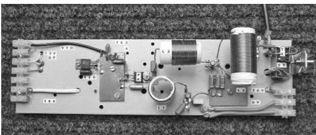
Fig 10.22: GW3UEP transmitter power amplifier
