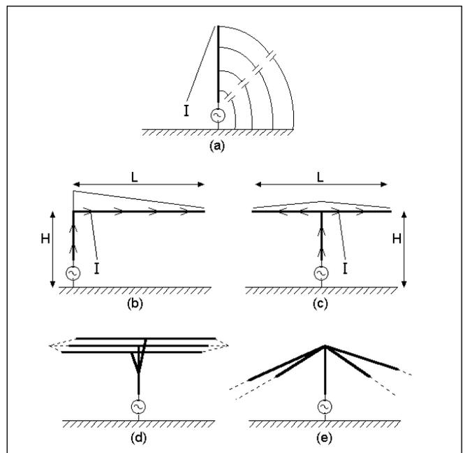
**Fig 10.33: (a) Cancellation of horizontally-polarised radiation from vertical. (b) Radiation pattern of short vertical antenna**
