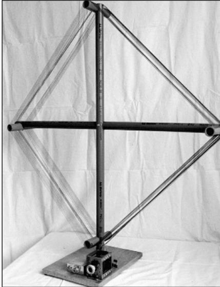
**(below) Fig 10.45:** 50-ohm preamp suitable for loop antennas
