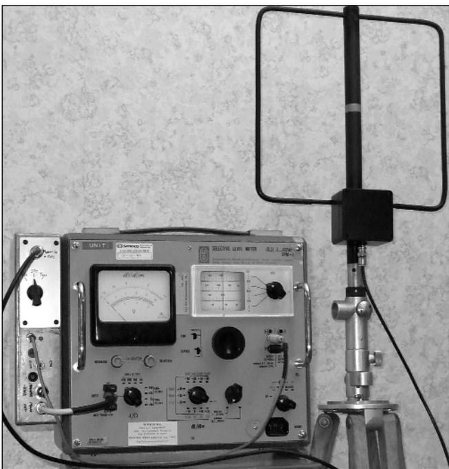
Fig 10.63: Field strength measuring system at M0BMU
