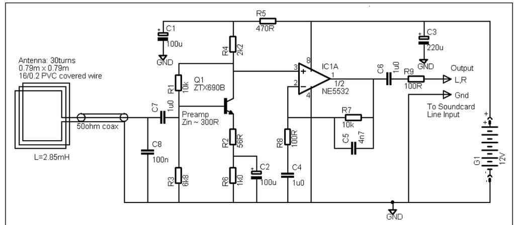
(above right) Fig 10.65: A VLF loop antenna together with pre-amplifier for use with an ordinary PC sound card. The input transistor, Q1 can be replaced by a BC337 with little change in performance
