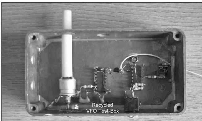
Fig 10.21: Ceramic resonator VFO for GW3UEP transmitter
