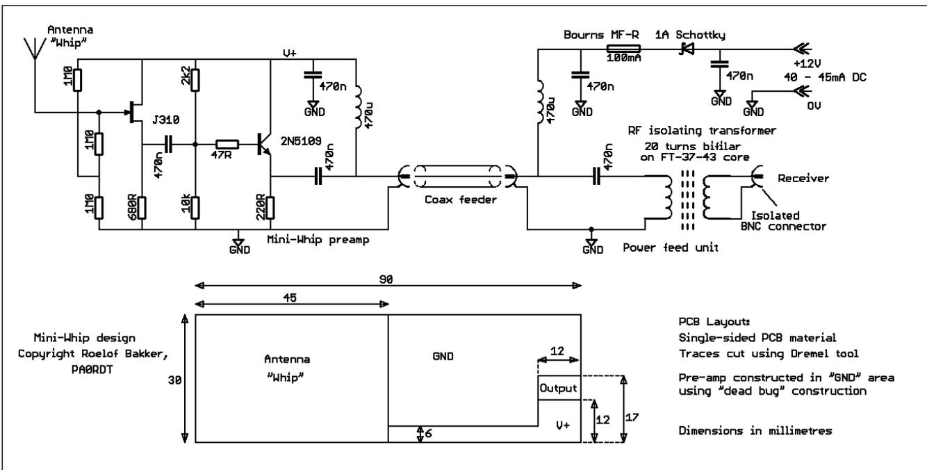
Fig 10.50: The PA0RDT-Mini-Whip®
