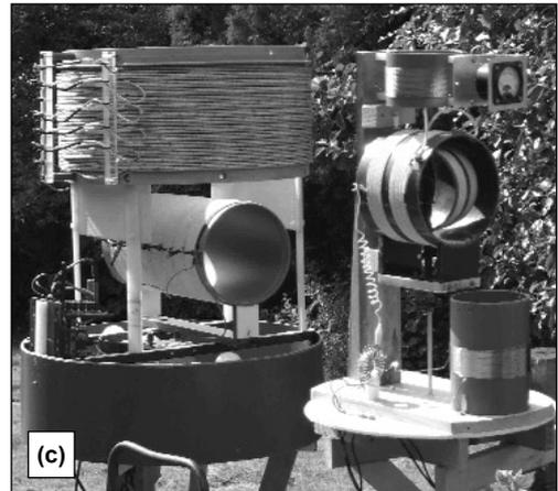
**Fig 10.38:** (a) LF antenna tuner; (b) Alternative antenna tuner circuit; (c) Antenna tuners at MOBMU using the circuit in (a) - 136kHz (left), 500kHz (right)
