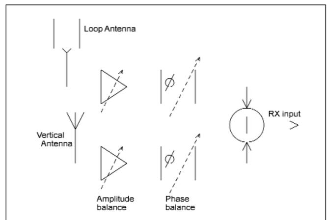
Fig 10.52: Loop/vertical directional array for low frequency reception
