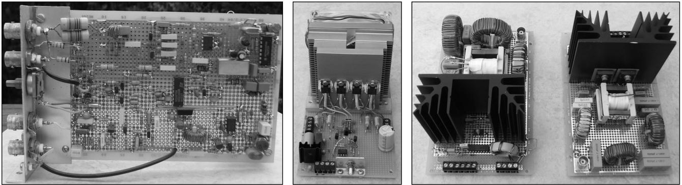
**Fig 10.23: Components of the EER transverter system: (left) Low-level transverter; (middle) Series modulator; (right) 136kHz and 500kHz power amplifiers**
