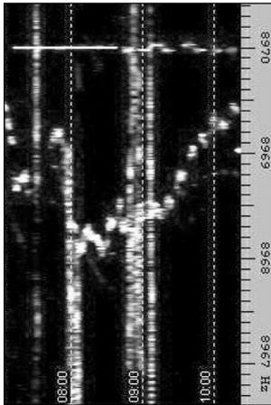
(above left) Fig 10.64: 8.97kHz signal from DK7FC received over a three hour period at MOBMU, together with local noise, in February 2011. The signal consists of a fixed carrier, followed by "FB" encoded in DFCW
