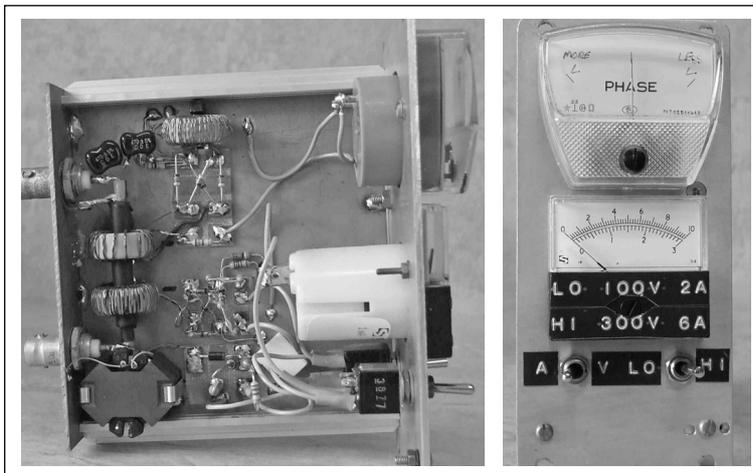
**Fig 10.62: LF tuning meter prototype**
