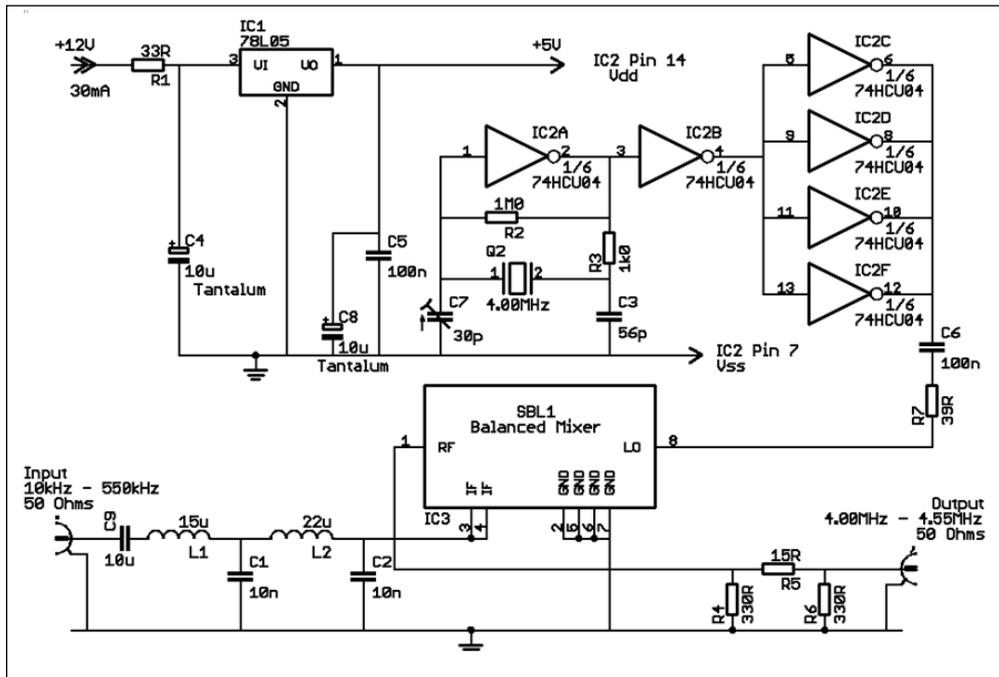
Fig 10.7: LF/MF - HF converter
