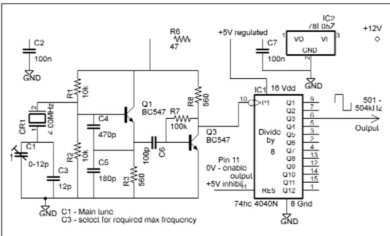
**Fig 10.29** shows a ceramic resonator VFO for 500kHz operation, using a 4MHz ceramic resonator with the oscillator frequency divided by eight. A similar design is used in the GW3UEP transmitter described above.
