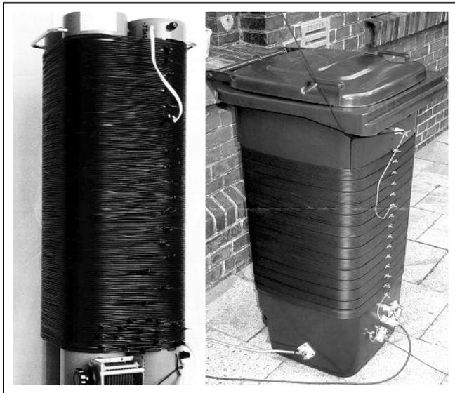
**Fig 10.40: Typical loading coils**
