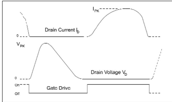
Fig 10.15: Class E waveforms
