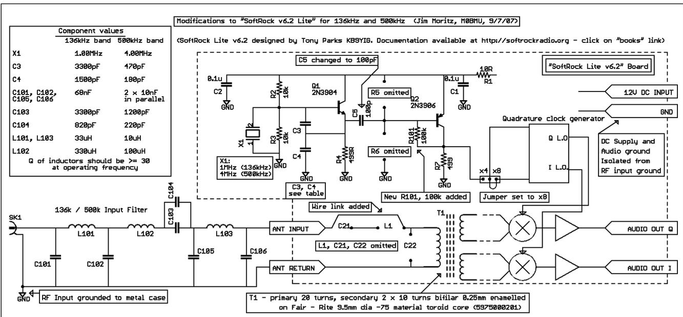
Fig 10.9: Modifications to SoftRock Lite v6.2 for 136kHz and 500kHz
