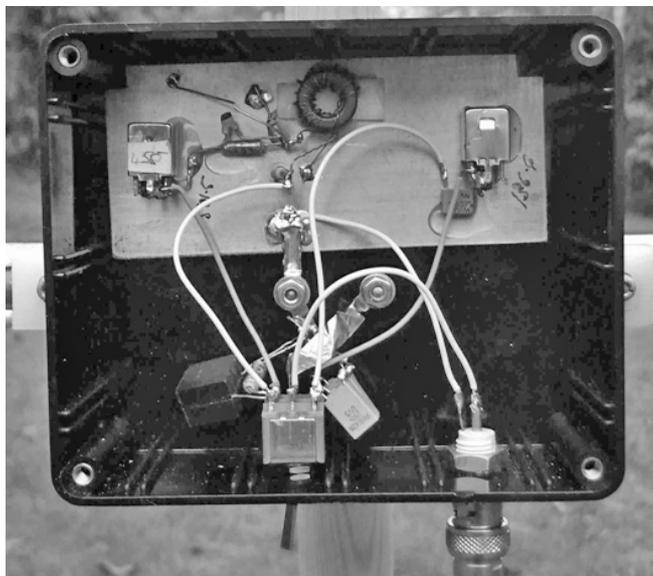
**(left / right) Fig 10.47:** Band-switched loop construction. The loop connections are the two bolts at the back of the case. The loop tuning capacitors C1 and C2 are mounted on the toggle band switch at the bottom
