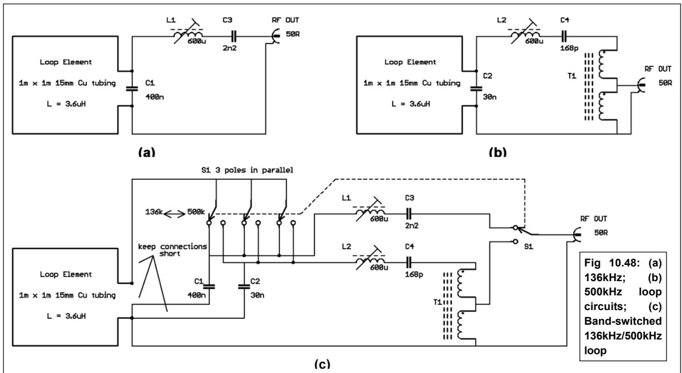
Fig 10.48: (a) 136kHz; (b) 500kHz loop circuits; (c) Band-switched 136kHz/500kHz loop
