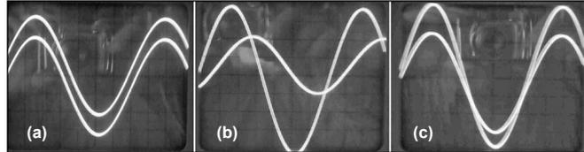
**Fig 10.60: Scopematch displays - upper trace voltage, lower trace current: (a) V and I in phase and equal magnitude; load is 50Ω resistive; (b) V lags I in phase, V less than I, so capacitive load of magnitude < 50Ω (about 20Ω here); (c) V and I in phase, but V greater than I, so resistive load >50Ω (about 80Ω here)**
