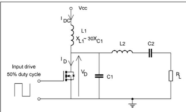
Fig 10.14: Basic class E PA circuit
