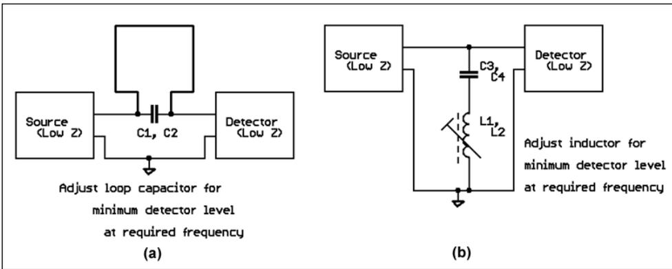
Fig 10.49: Adjusting resonant frequency of (a) loop, (b) auxiliary tuned circuit
