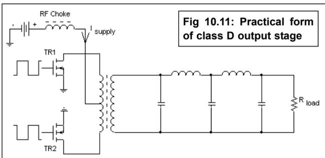
**Fig 10.11: Practical form of class D output stage**
