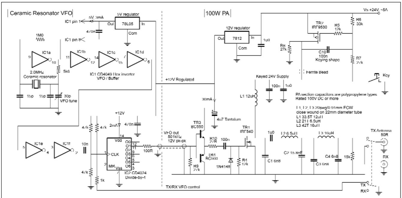
**Fig 10.20:** GW3UEP 100W 500kHz transmitter
