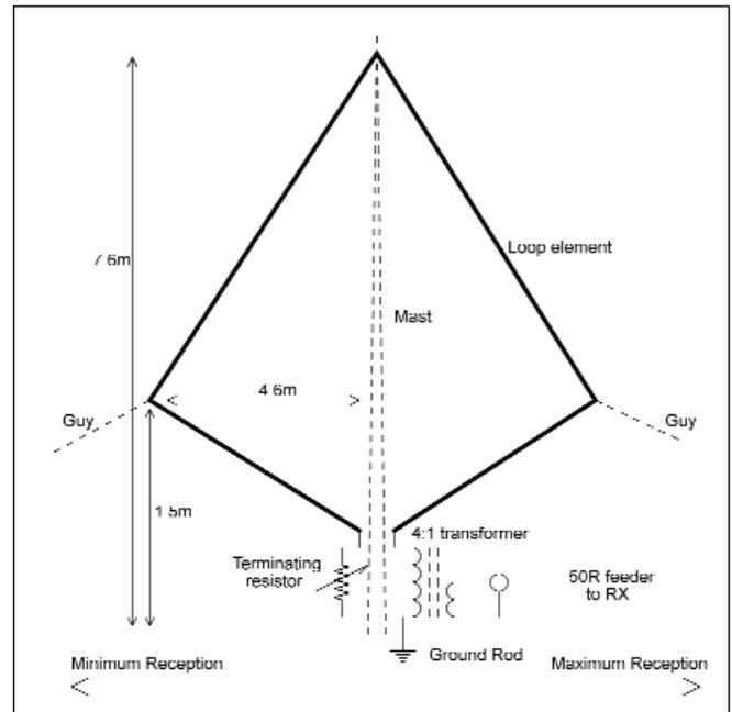
Fig 10.51: Single K9AY loop for LF/MF use
