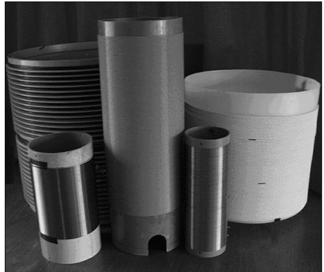
**Fig 10.41: Some of the loading coils of Table 10.4**
