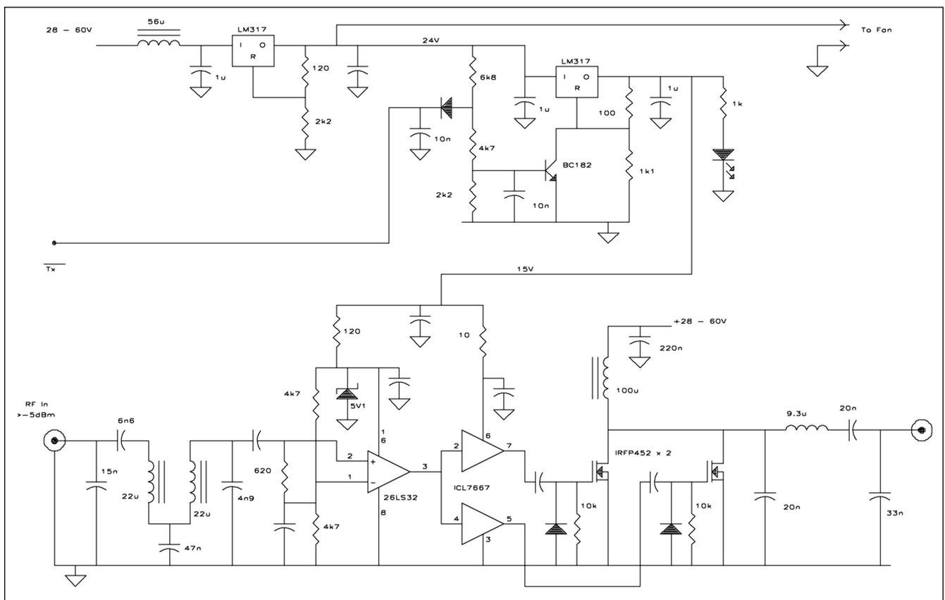
**Fig 10.17:** G4JNT QRO class E 500kHz PA. All unmarked capacitors are 100nF. Diodes are 1N4145
