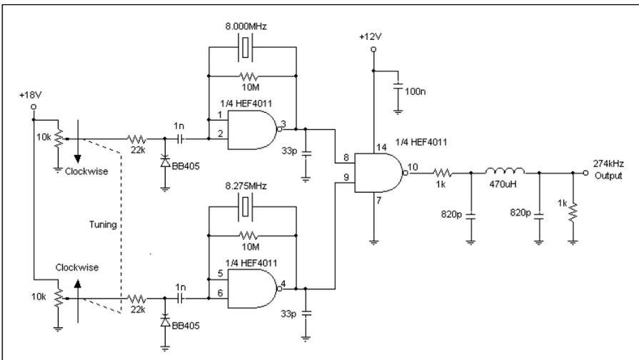
**Fig 10.30: 'Crystal mixer' VFO from GOMRF transmitter**
