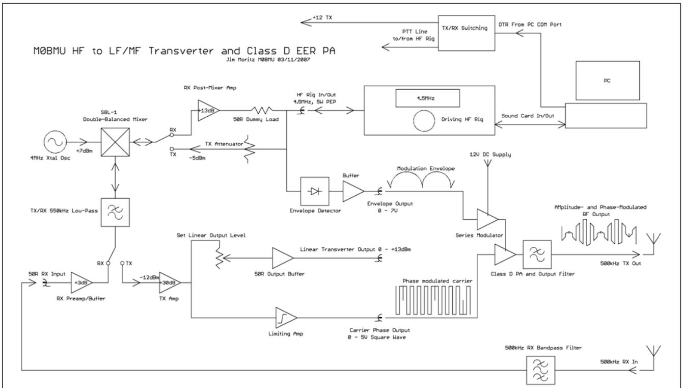
**Fig 10.24: EER Transverter block diagram**
