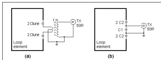
**Fig 10.43: Transmitting loop matching circuits**
