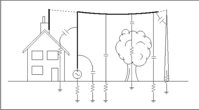
**Fig 10.35: Loss in the environment around an antenna**
