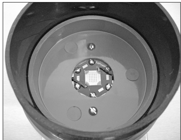
Fig 11.168: The extreme beacon LED mounted in one of the now-standard housings
