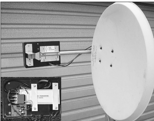
Fig 11.18: Quickstarter for 3cm mounted on the feed arm of a surplus TVRO offset dish
