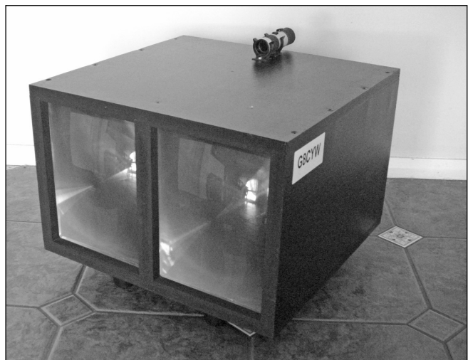
Fig 11.173: The Fresnel lens rig, suitable for a transmitter and receiver, or a transceiver and beacon
