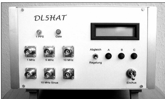
Fig 11.43: Picture of the prototype high precision frequency standard for 10MHz controlled by GPS
