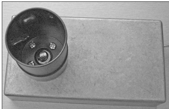
Fig 11.145: The completed AM receive head, showing the photo diode and mounting tube
