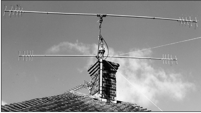
Fig 13.44: A compact two-element multiband beam
